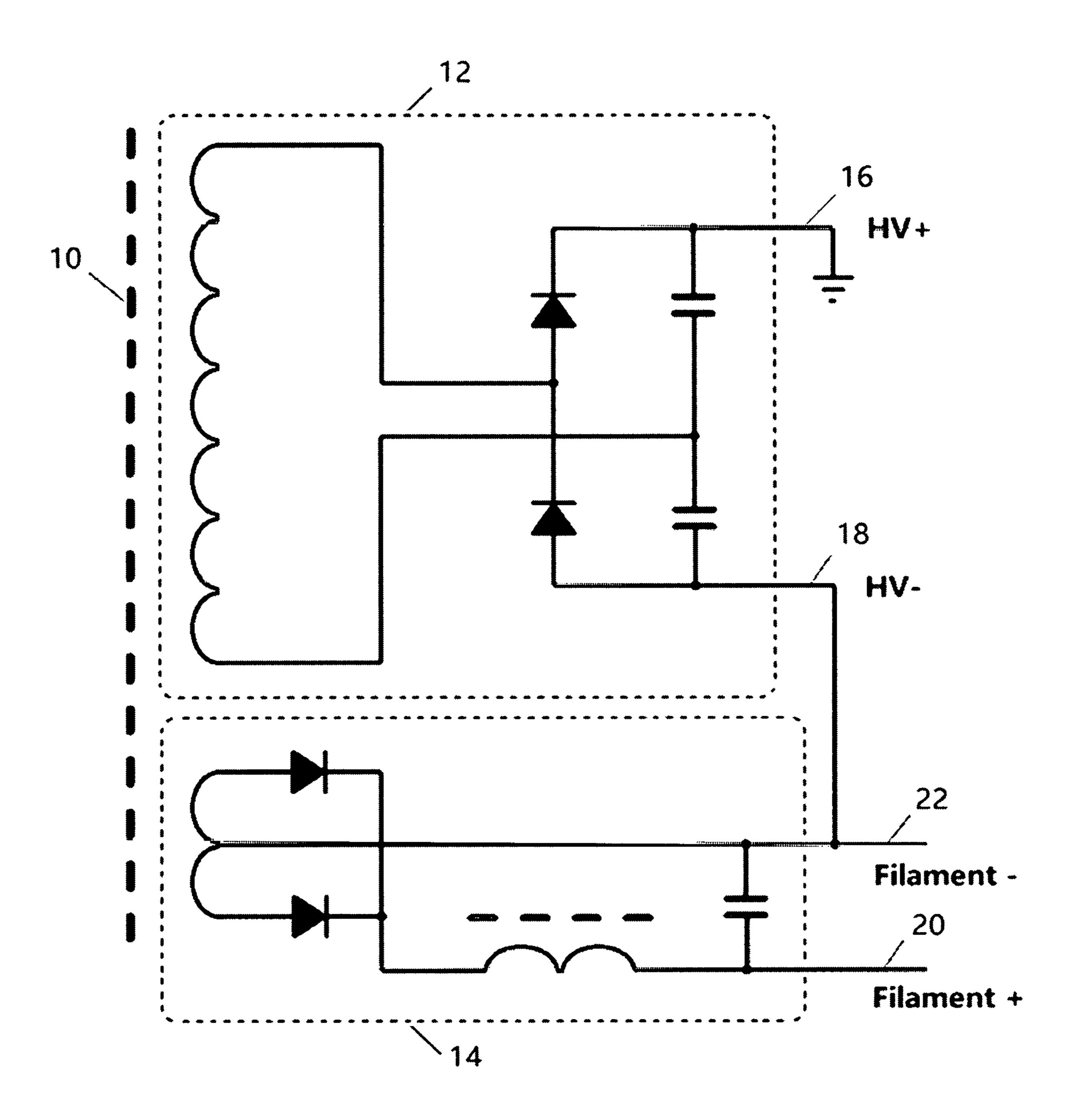
Figure 1 The secondary winding circuit of the main transformer in an iMOT power supply
