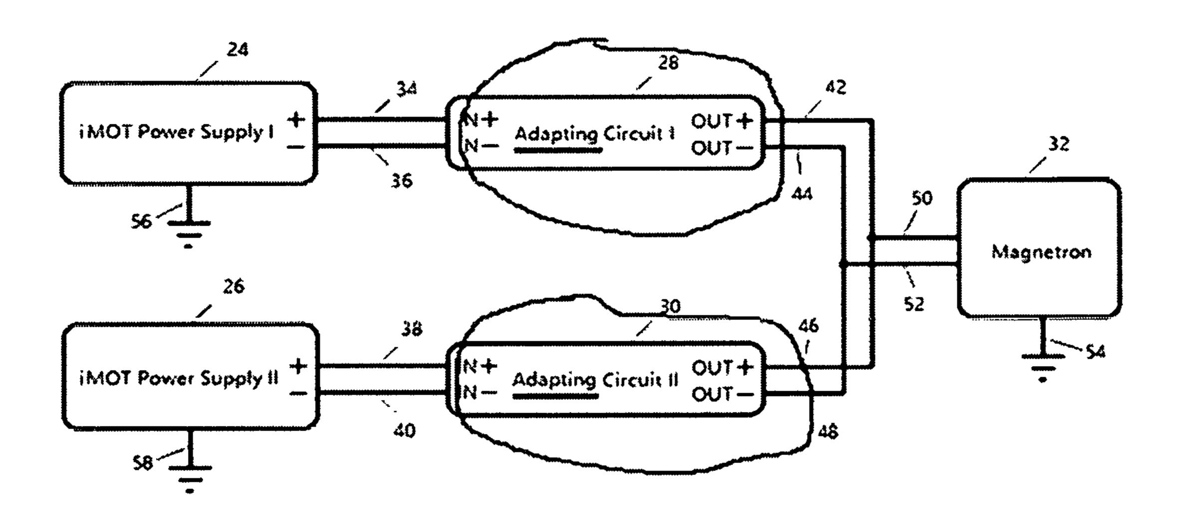
Figure 2 Two iMOT Power Supplies are connected with the Adaptingve Circuits for Driving One Magnetron
