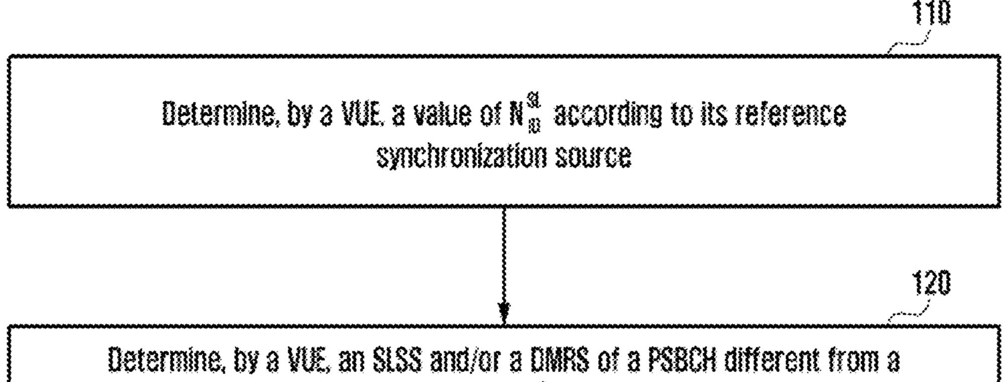
Determine, by a VUE, an SLSS and/or a DMRS of a PSBCH different from a D2D system according to the value of N<sub>10</sub>, wherein the SLSS comprises a PSSS and an SSSS, and the DMRS of the PSBCH is determined by a DMRS sequence and an orthogonal mask of the PSBCH
