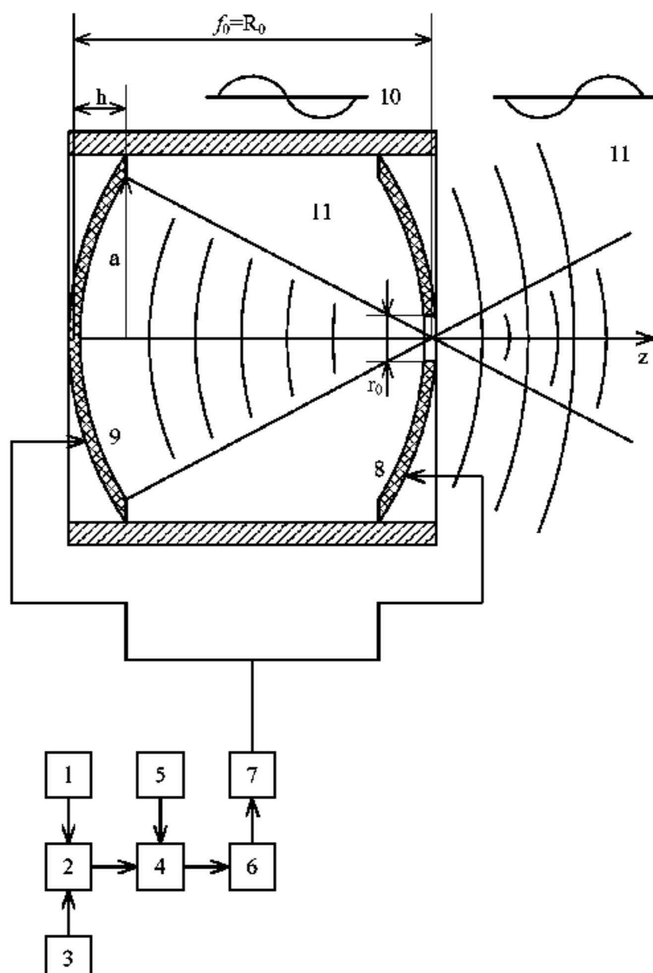
with convex aperture is made with an open axial hole with radius  $r=(2\div 3)\times r_0$  in the central part of the convex spherical surface of the aperture.
