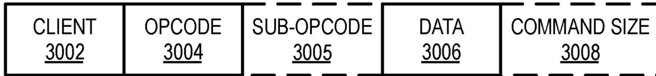
FIG. 30B GRAPHICS PROCESSOR COMMAND SEQUENCE
