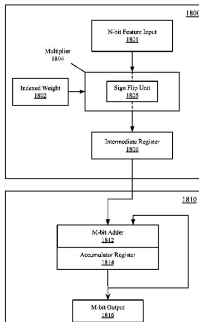
product to a value stored in the accumulator register and update the value stored in the accumulator register.
