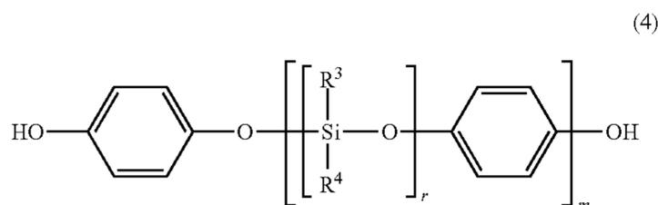
wherein  $\text{R}^3$  and  $\text{R}^4$  are identical to those described above. The average chain length of the polyorganosiloxane block represented by the general formula (4) is  $(r \times m)$ , and the range of the  $(r \times m)$  is the same as that of the "n".
