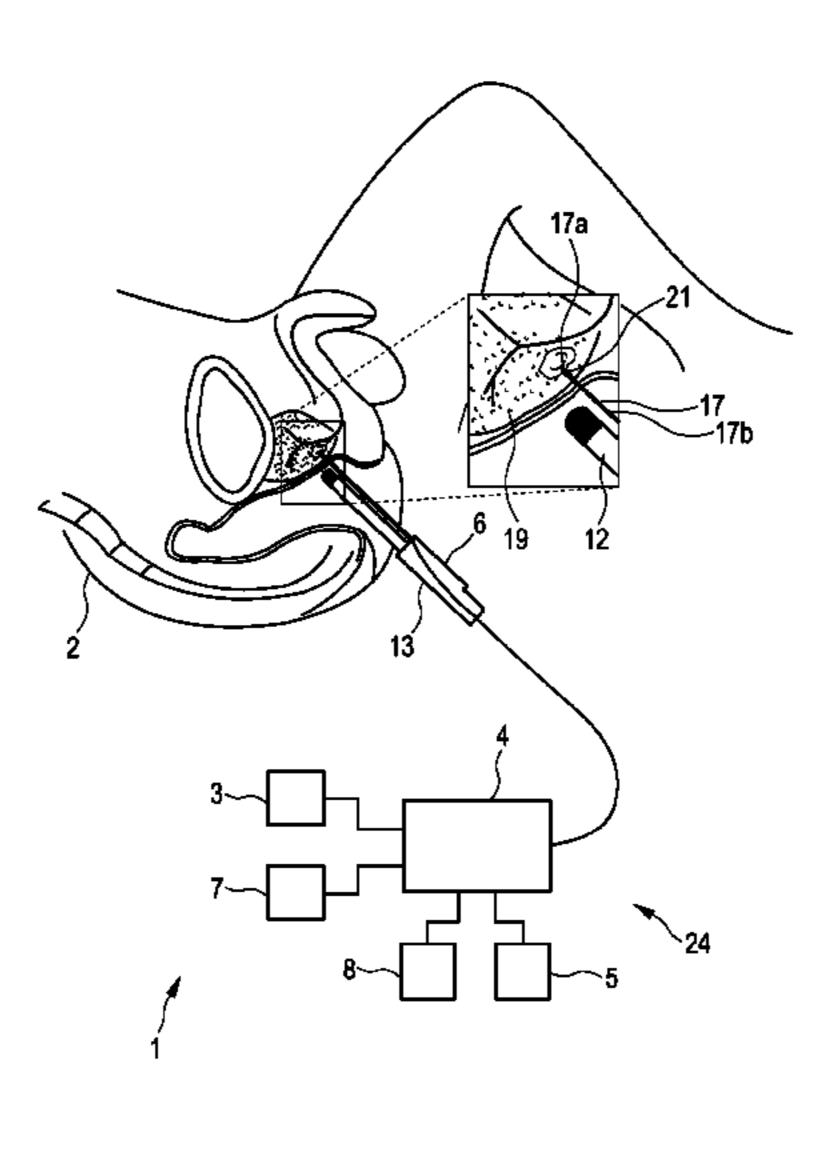
imaging unit (4) generates an indicator image showing the inner part (19) and an indicator of the introduction element (17) based on the tracked location. A display (5) displays the indicator image providing feedback about the location of the introduction element (17).
