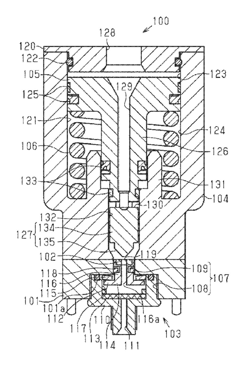
cates in the same direction as a direction in which the valve element reciprocates in the primary pressure chamber. As a difference between the primary pressure and the secondary pressure increases, the valve seat moves toward the secondary pressure chamber.
