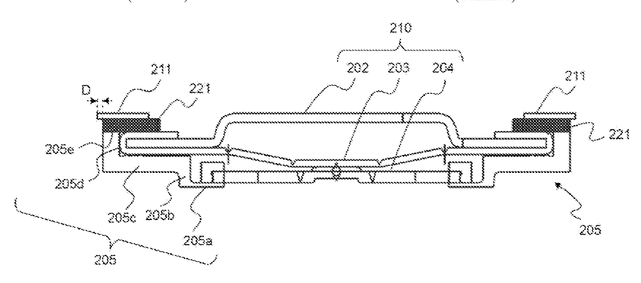
assembly and the cylindrical battery case; and a washer for fixing the cap assembly to the cylindrical battery case, the washer coupled to an upper surface of an outer circumferential portion of the open upper end of the cylindrical battery case.
