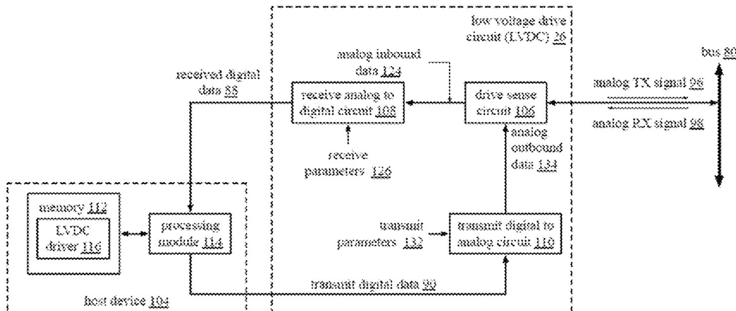
bined with the oscillating component to produce the analog outbound data. A drive sense circuit drives an analog transmit signal onto a bus, wherein the analog outbound data is represented within the analog transmit signal as variances in loading of the bus in a first frequency range and wherein analog inbound data is represented within an analog receive signal as variances in loading of the bus in a second frequency range.
