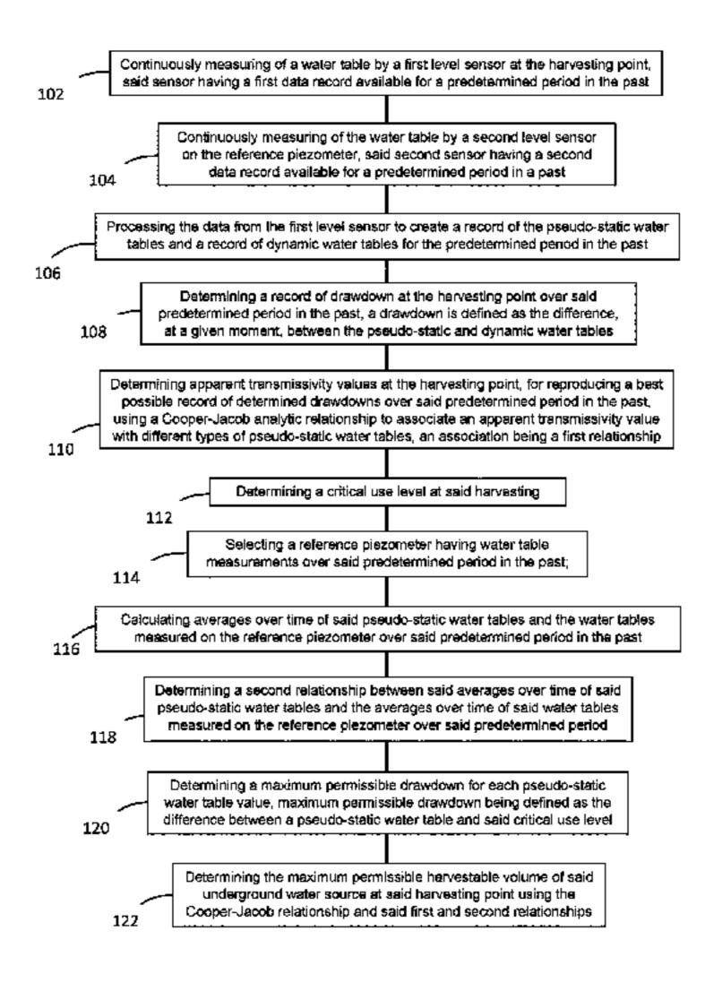
on the removal point, the sensor having a first log of available data over a predetermined period that has passed; and another continuous measurement by a second piezometric level sensor on the reference piezometer, the second sensor having a second log of available data over the predetermined period that has passed; the method also comprising subsequent steps implemented by a calculation machine.
