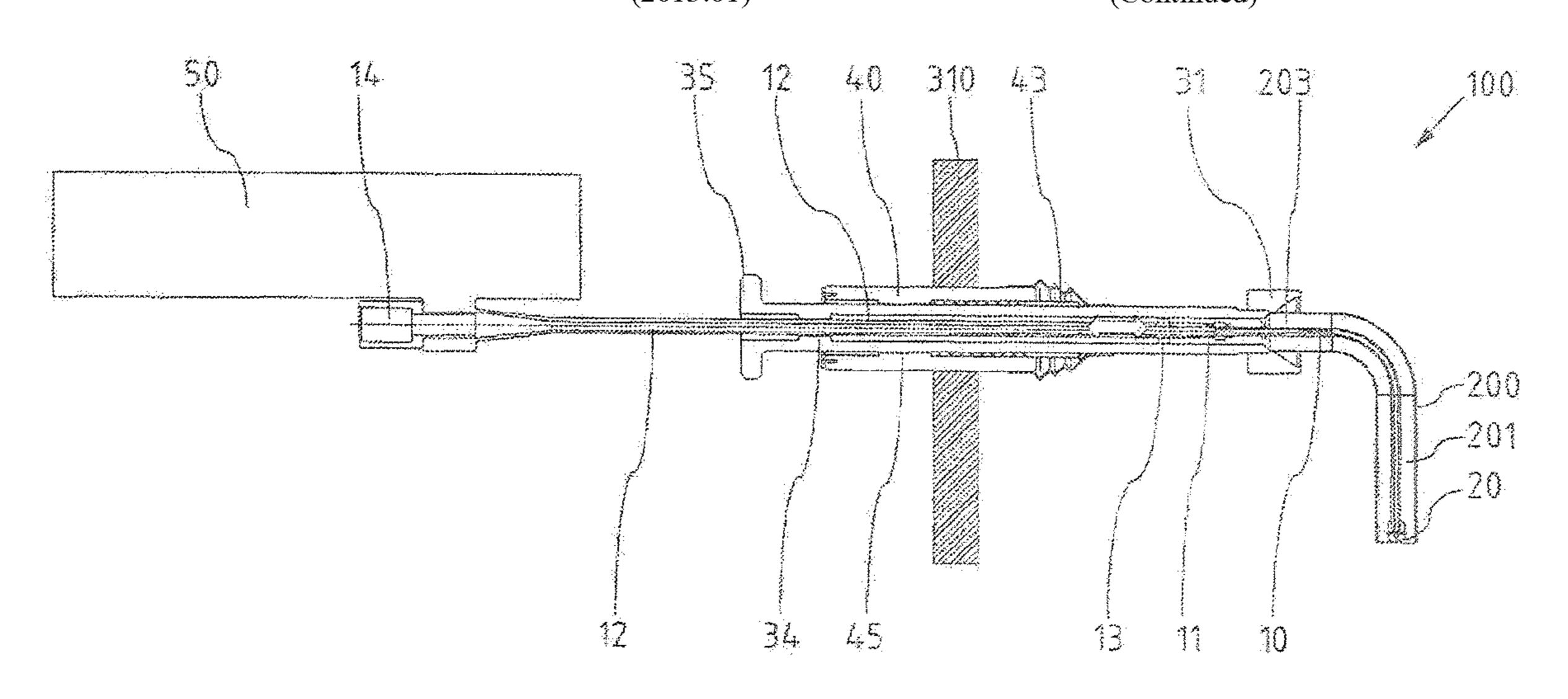
processed. The blasting abrasive feed hose (10) is guided in a supporting element (30) and this element (30) is guided in a displaceable manner in a stationary bearing element (40).
