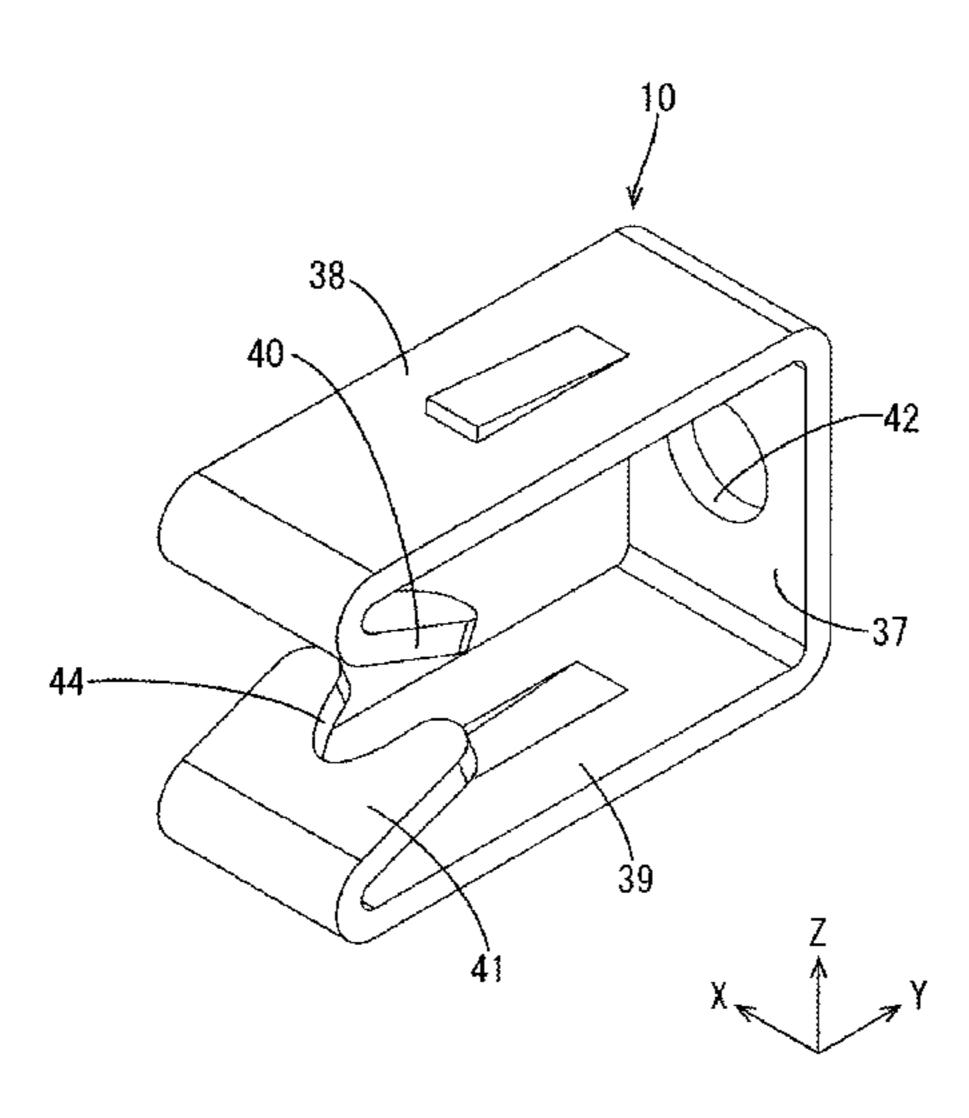
end edges of the front wall, and that are to be disposed around the insulating covering; and an upper holding portion and a lower holding portion that protrude from rear end portions of the upper extending piece and the lower extending piece toward the insulating covering, and that clamp an outer surface of the insulating covering, wherein at least the upper and lower extending pieces and the upper and lower holding portions are made of a metal.
