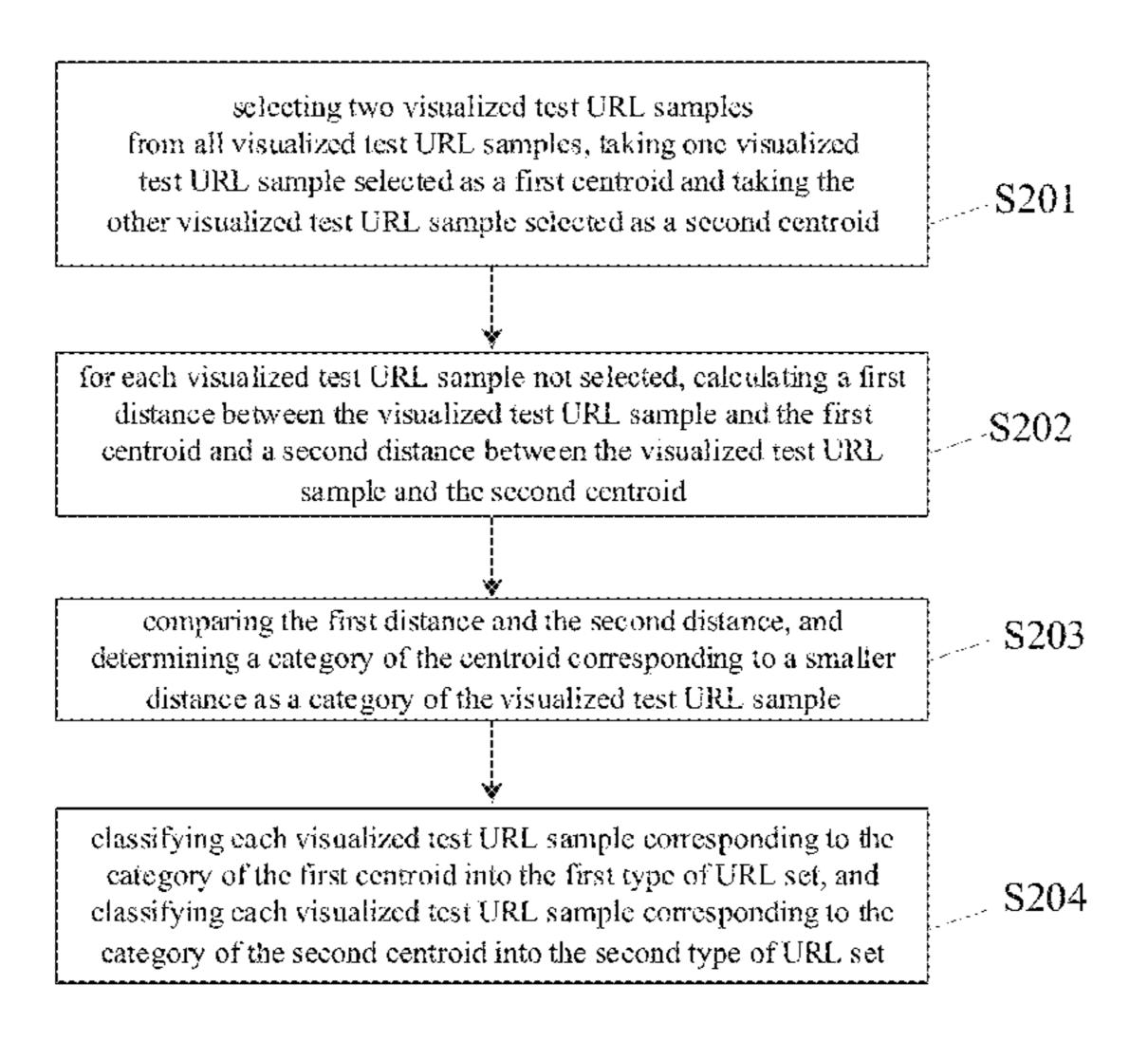
URL sets; comparing sample sizes of the first type and second type of URL sets, determining the URL set with a larger sample size as a normal URL set, and determining the URL set with a smaller sample size as an abnormal URL set.
