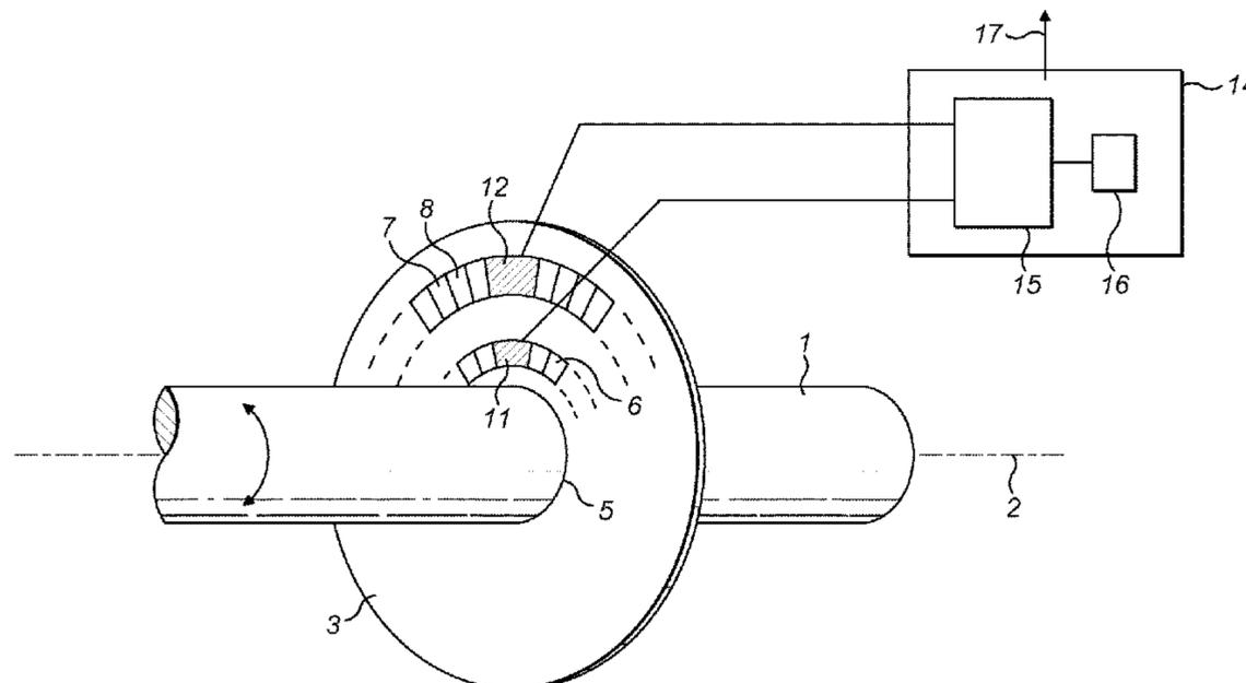
ring by a predetermined distance; and if p and q are co-prime: selecting j to be p and k to be q; and assembling the position sensing arrangement by mounting the disc to the articulated structure such that both the disc and the revolute joint are permitted to rotate about the same axis.
