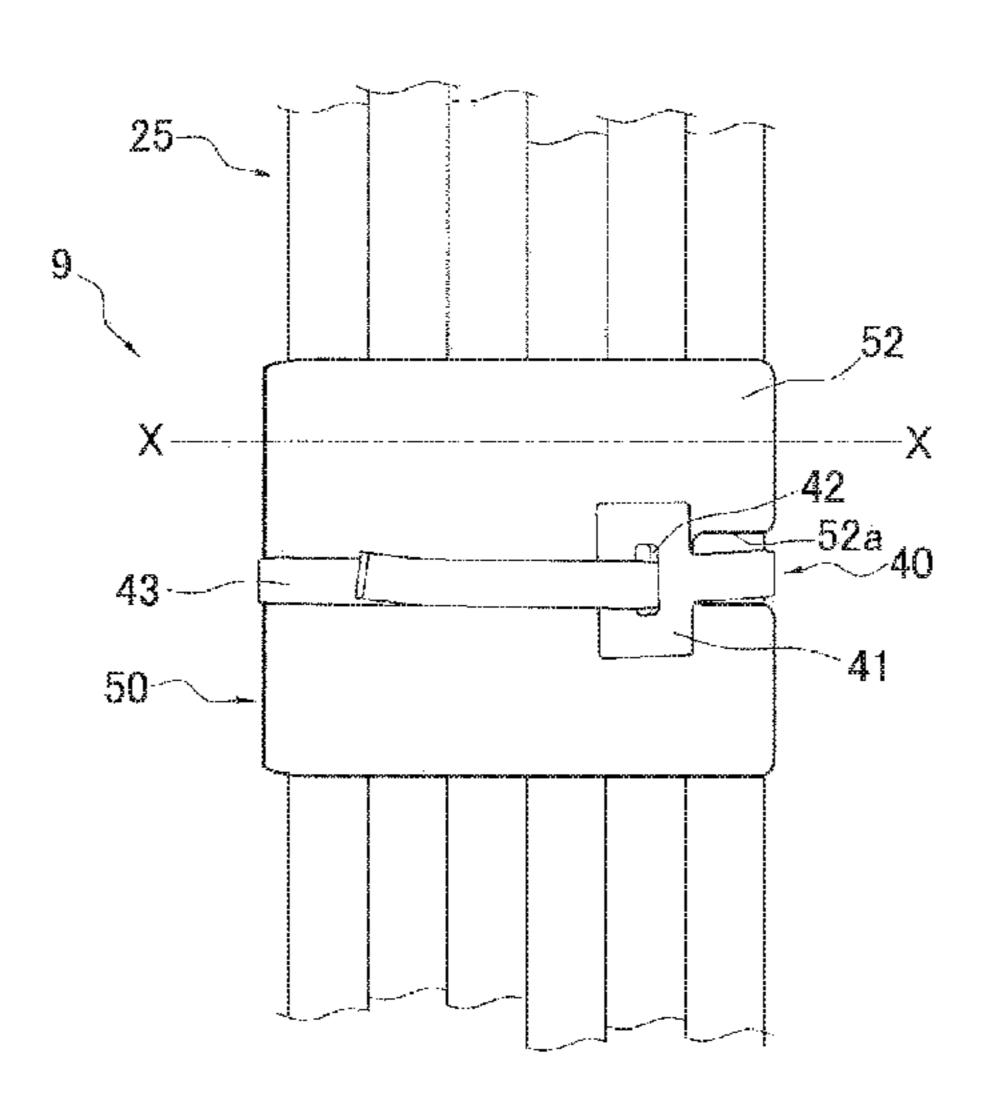
opposite side of a main body portion side anchored in the anchoring portion. The bundling component is made of aluminum or aluminum alloy. At least part of the bundling component and at least part of the plurality of members are secured to each other with a brazing material interposed between the parts.
