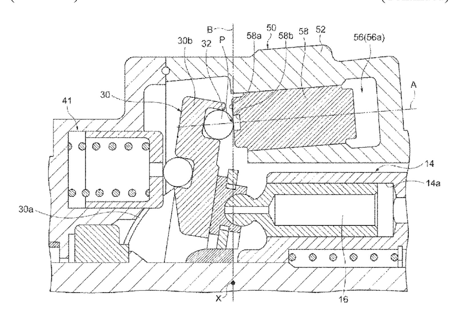
is pressed toward the swash plate by the piston portion, in which when the inclination angle of the swash plate is an intermediate inclination angle in which the discharge capacity of the working fluid becomes an intermediate amount between the maximal amount and the minimal amount, a contact point between the piston portion and the pressed portion is located at a center portion including an axis center of the piston portion in an end surface on the side of the swash plate in the piston portion.
