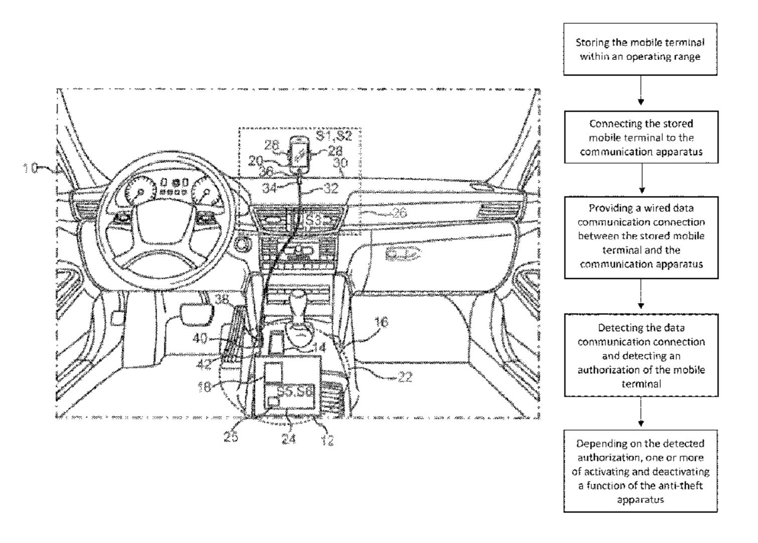
detects whether the data communication connection has been established with the mobile terminal by the connecting device and detects whether the mobile terminal is authorised to operate the anti-theft system, and depending on whether the authorisation has been detected, activates and/or deactivates a function of the anti-theft system.
