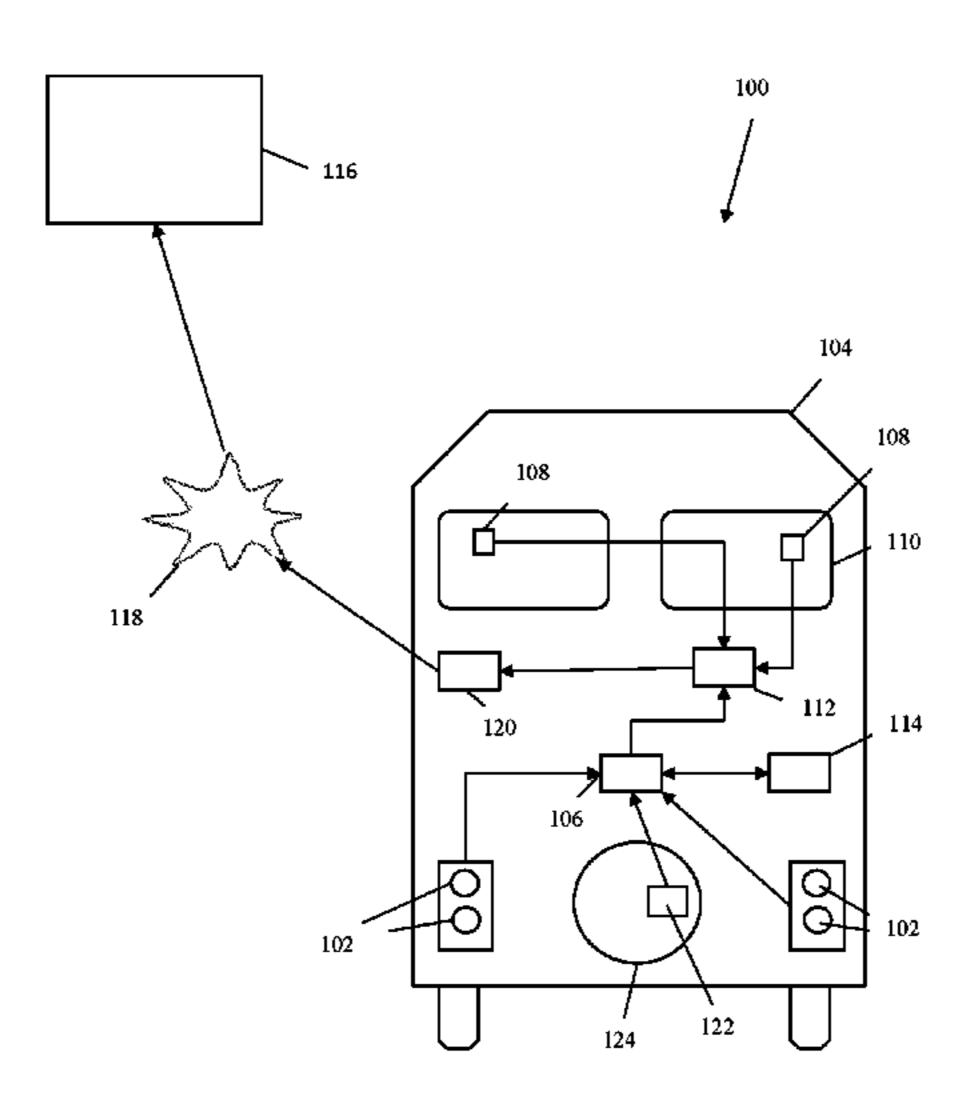
the object. The system is arranged to automatically make the captured image available for inspection in response to the trigger determiner determining that the characteristic of the impact is greater than the predefined threshold value so that the object in the image can be identified substantially in real-time.
