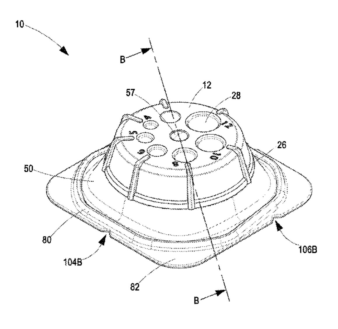
tapering radially inwardly from the planar surface portion of the base towards the contact lip, which in use biases the contact lip into sealing engagement with the target object to efficiently collect dust and debris, with substantially the entire planar support surface portion contacting the target object thereby to provide a stability for drilling straight holes.
