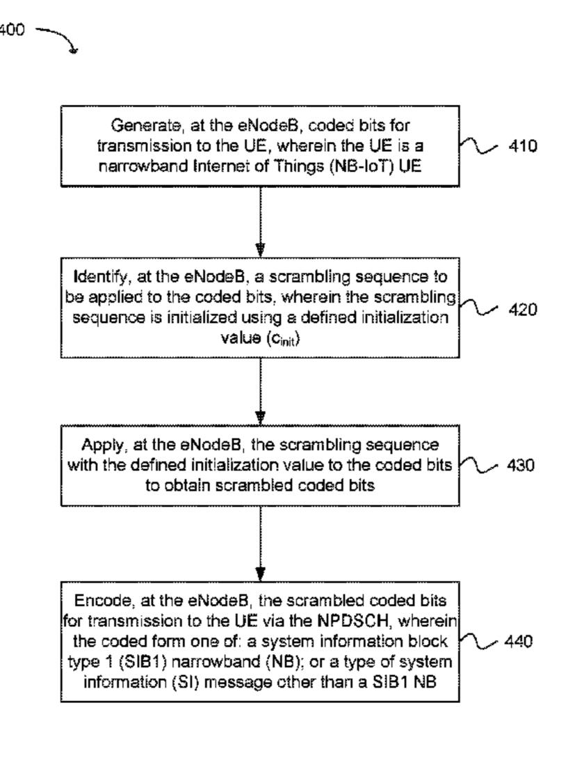
the coded bits to obtain scrambled coded bits. The eNodeB can encode the scrambled coded bits for transmission to the UE via the PDSCH.
