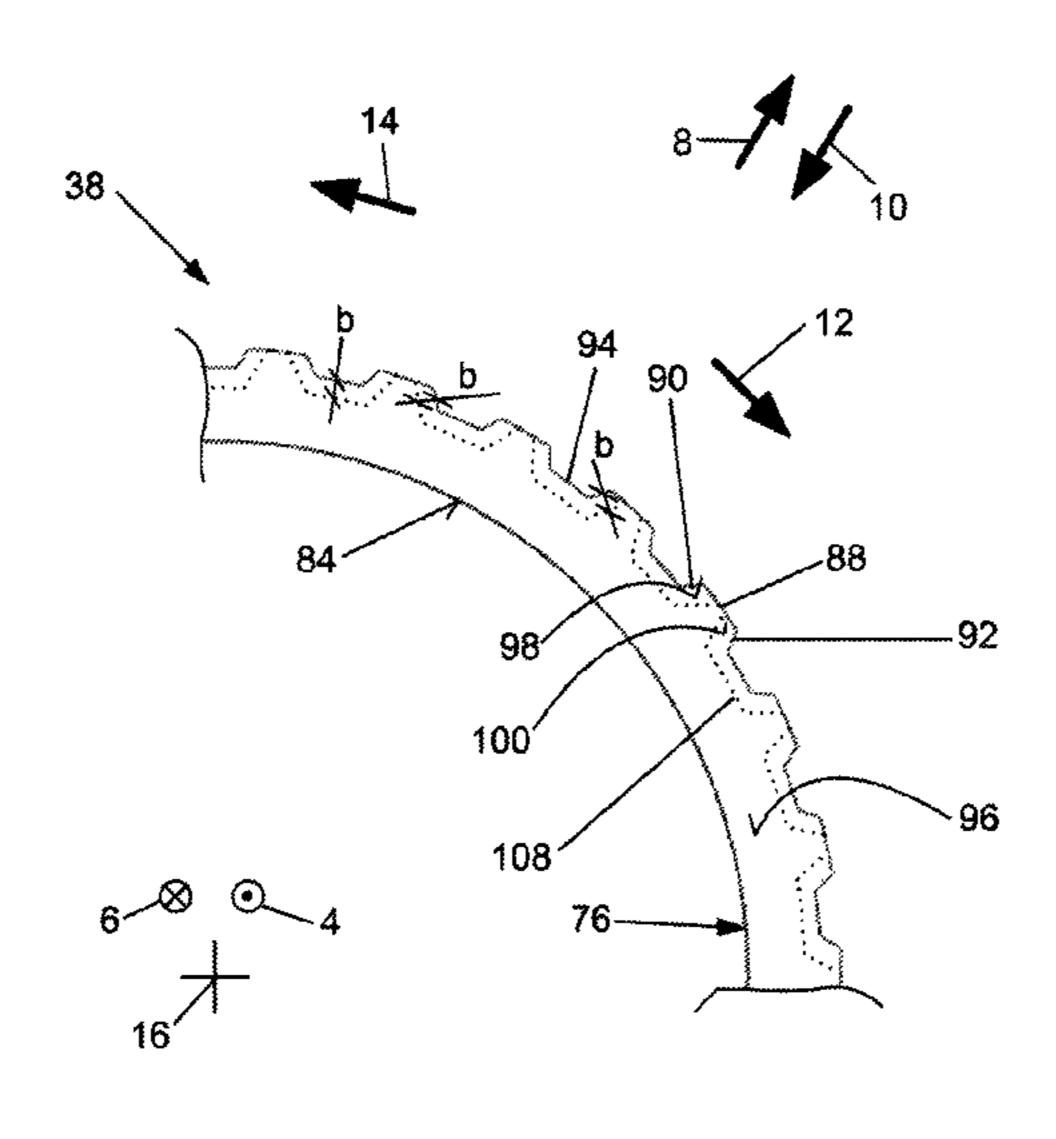
base element (76) has at least one hardened region (96) in which the base element (76) is designed as harder than in the tooth flank regions (98, 100) of the teeth (80). In addition, the disclosure relates to a disk clutch (26) with such a disk (38), a double clutch device (2) with such a disk clutch (26), and a method for producing such a disk (38).
