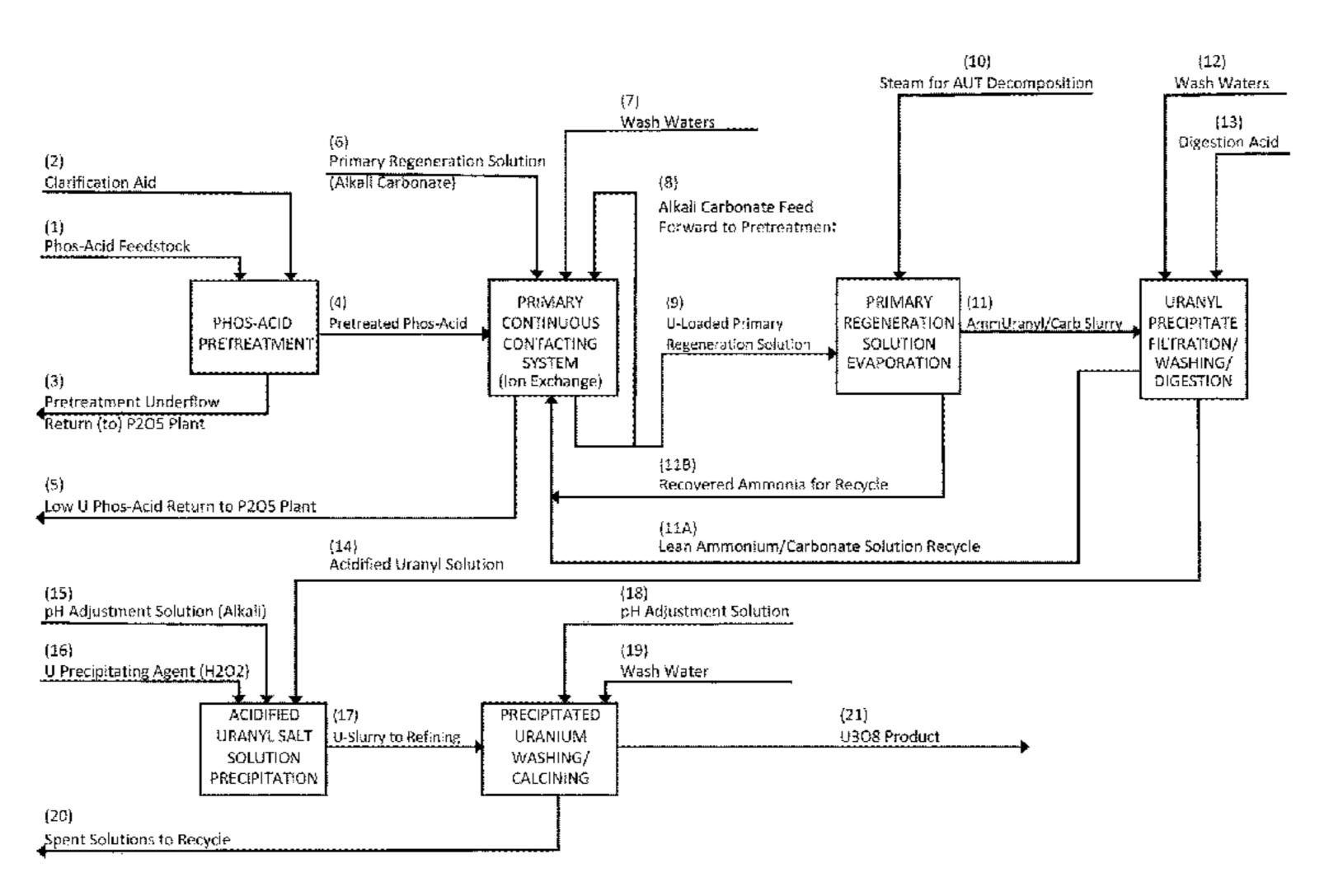
carbonate and produce an intermediate uranium carbonate/ oxide solid material. These solids are digested in an acid medium, and then processed in the same manner as the secondary regeneration solution from the dual cycle process to produce an intermediate uranyl peroxide that is calcined to produce a final uranium oxide product.
