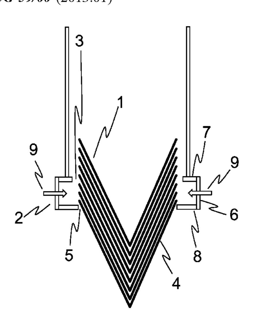
stack into the chamber (2) from above the chamber (2); and allowing the lowermost cone sleeve (4) to sit within the lower circular opening (5) and allowing the cone sleeves above the lower-most cone sleeve (4) to protrude from the top of the chamber (2) characterized in that pressurized gas is introduced into the chamber via the inlets (9) thereby to create an elevated pressure within the chamber (2).
