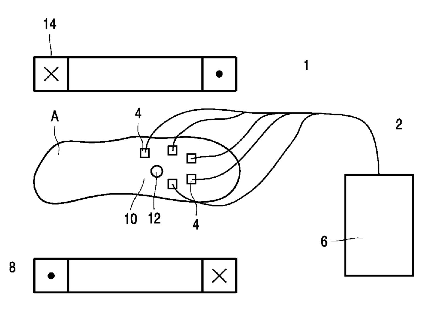
signals to obtain information about the spatial distribution of the magnetic particles in the examination area; and determining a conductivity in the examination area as a function of a magnetization status of the magnetic particles.
