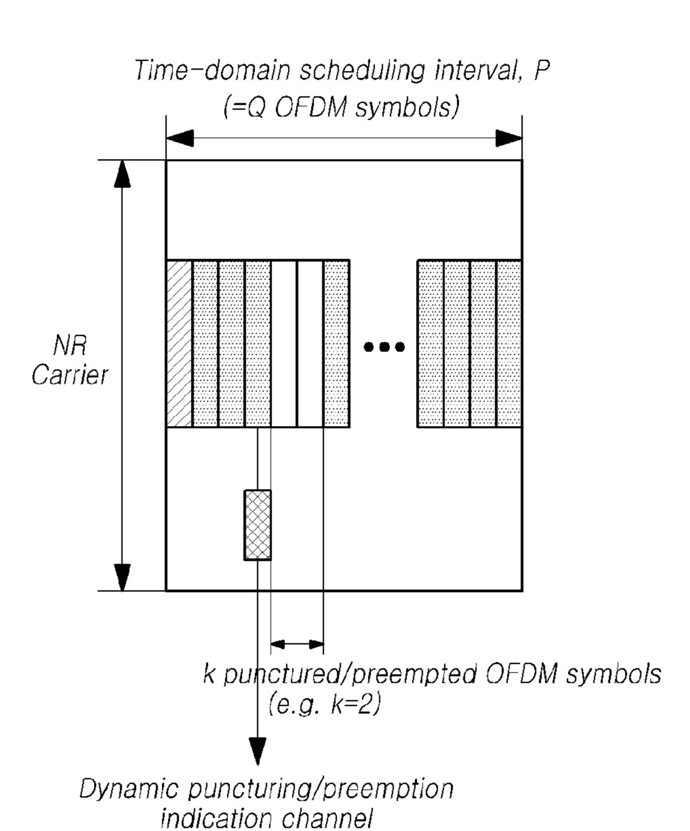
Case b. out-band dynamic puncturing/preemption indication channel transmission
