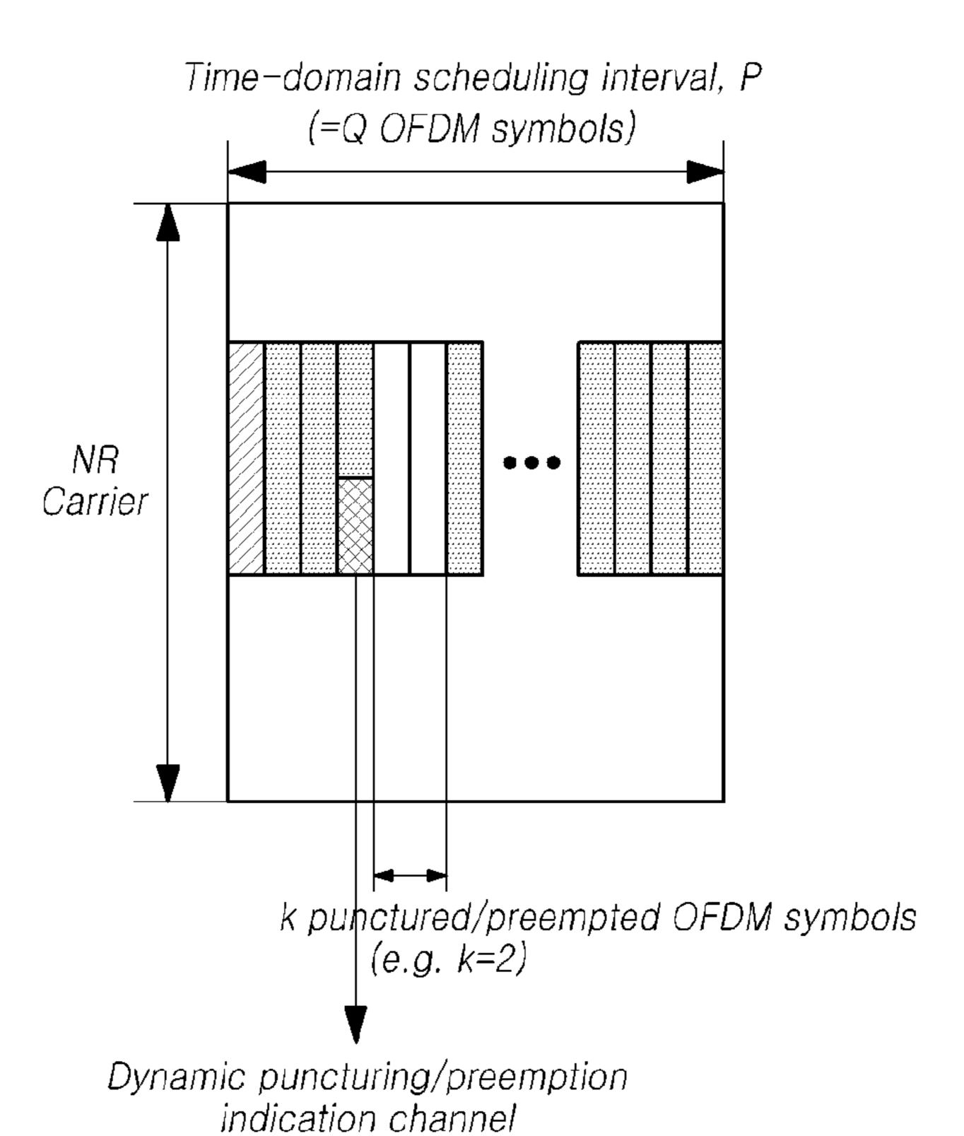
Case a. in-band dynamic puncturing/preemption indication channel transmission
