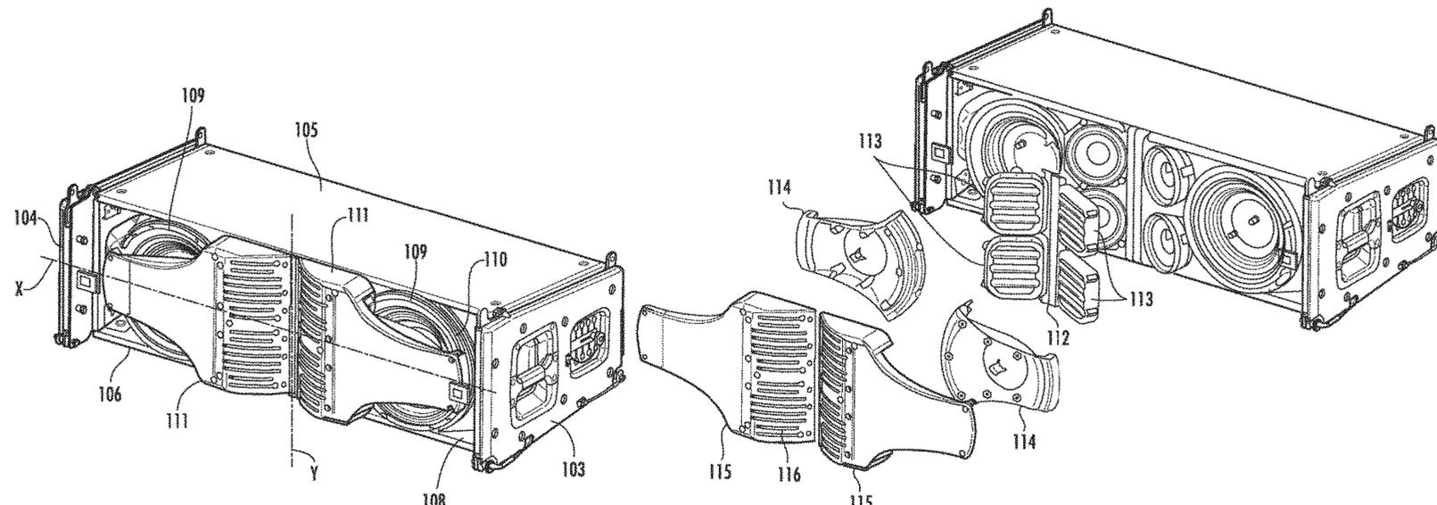
waveguide attached to at least one integrator. The at least one integrator may include at least one plug and at least one lens.
