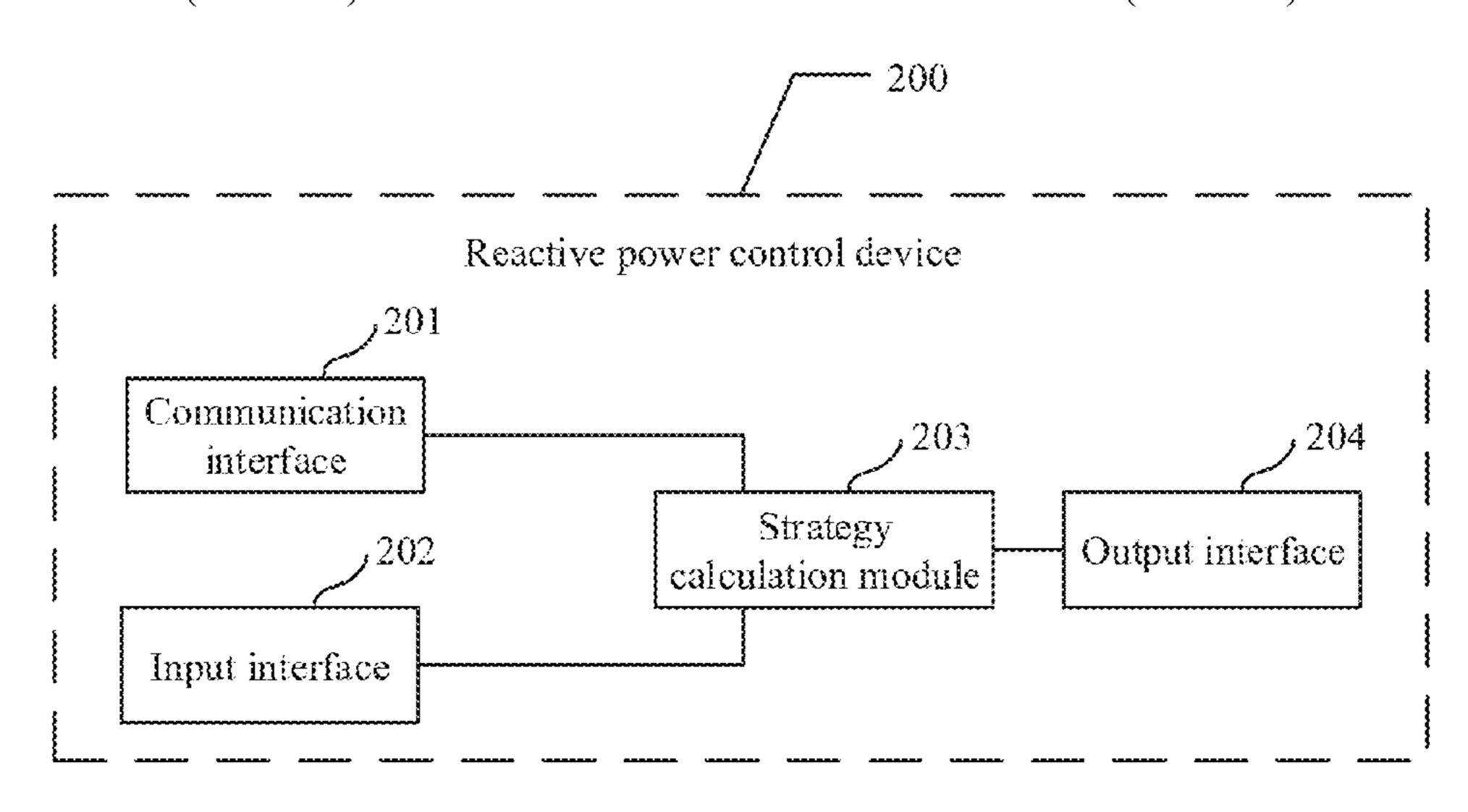
electrical quantity parameter, and allocate reactive power to be provided by a regulatable reactive device based on the target reactive power value; and an output interface, configured to send a command for providing the allocated reactive power to the regulatable reactive device.
