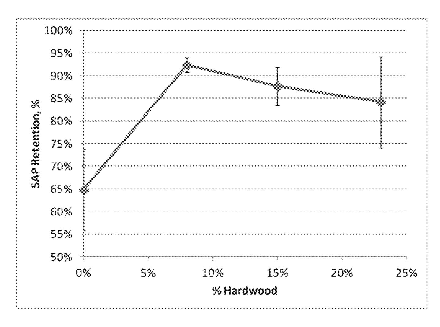
Procedure: Form pad with 50% fluff pulp and 50% SAP. Shake pad on mesh screen. Determine SAP retained by weight difference before and after shaking.
