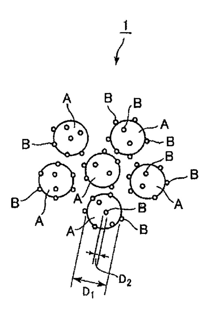
when, in the powder mixture, the total weight of the ceramic powder A to be used whose prescribed particle diameter  $D_1$  is  $W_1$ , and the total weight of the ceramic powder B to be added to the ceramic powder A is W2, an addition ratio Y of the ceramic powder B defined by  $Y=W_2/(W_1+W_2)$  satisfies:  $Y \ge 0.2066 \times D_1^{-0.751}$  and  $Y \le 0.505 \times D_1^{-0.163}$ .
