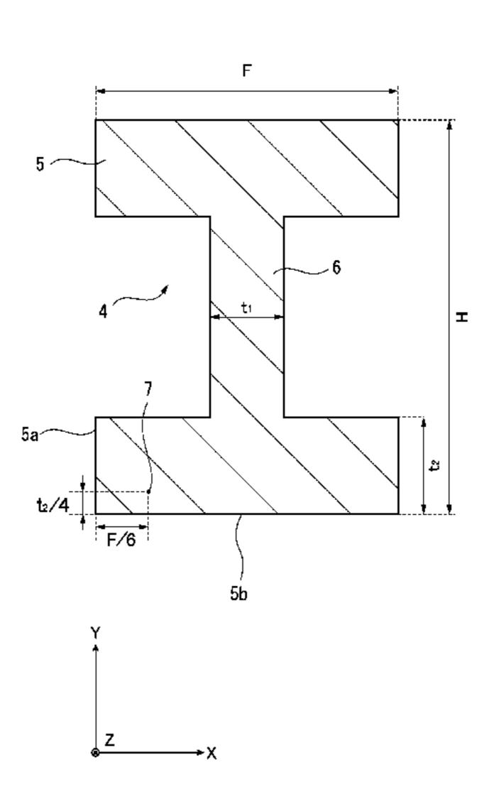
direction of the flange at a position separated in the width direction of the flange from the end face in the width direction of the flange by (1/6)F; and the absorbed energy in a Charpy test at the measurement position 7 at -20° C. is 200 J or more.
