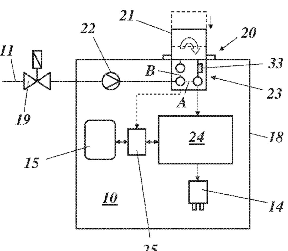
machine via the fixed water connection flows through the cartridge and is thereby filtered and/or enriched with additives.
