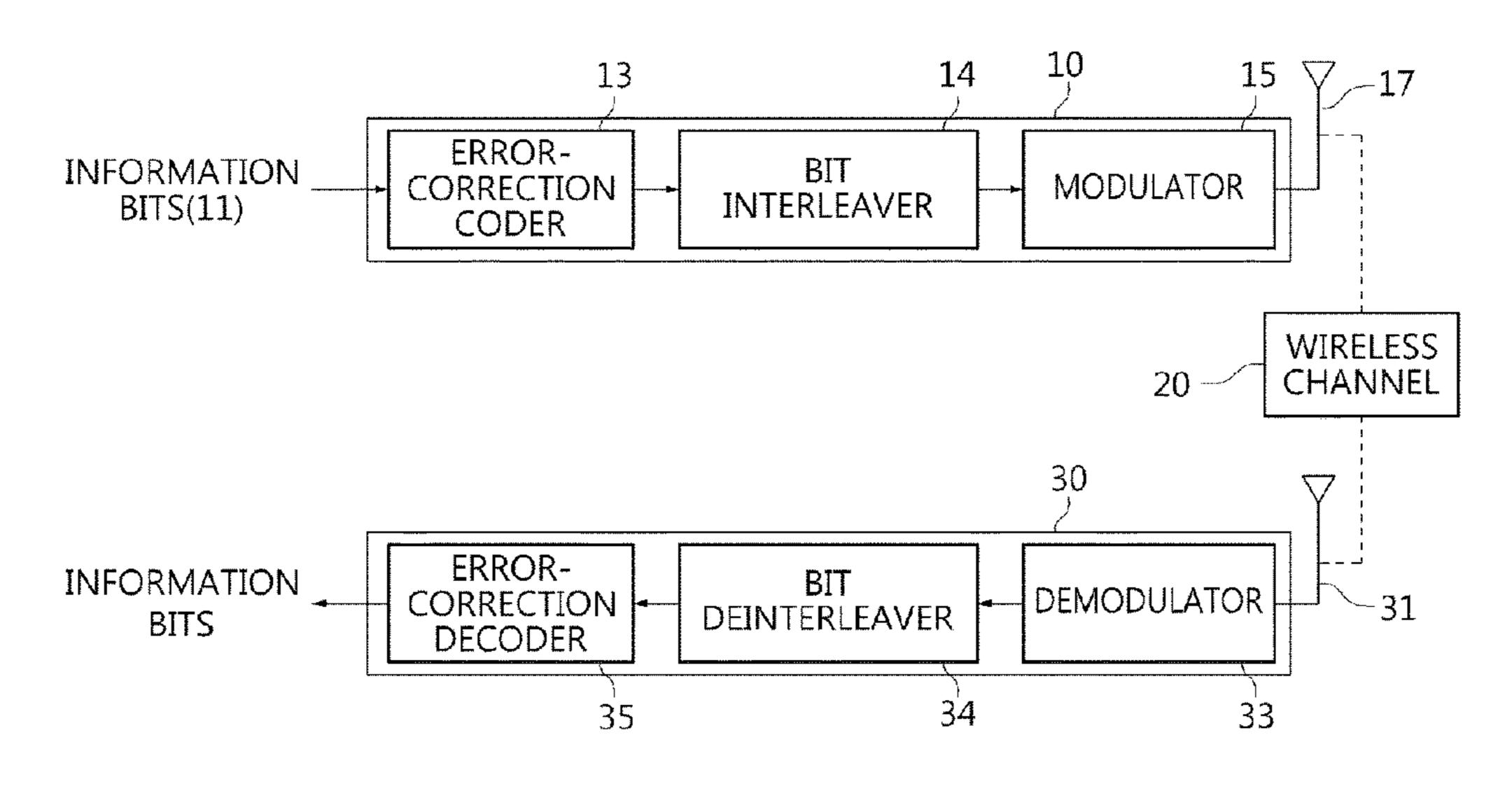
to a parallel factor of the LDPC codeword. The second memory provides the interleaved codeword to a modulator for quadrature phase shift keying (QPSK) modulation.
