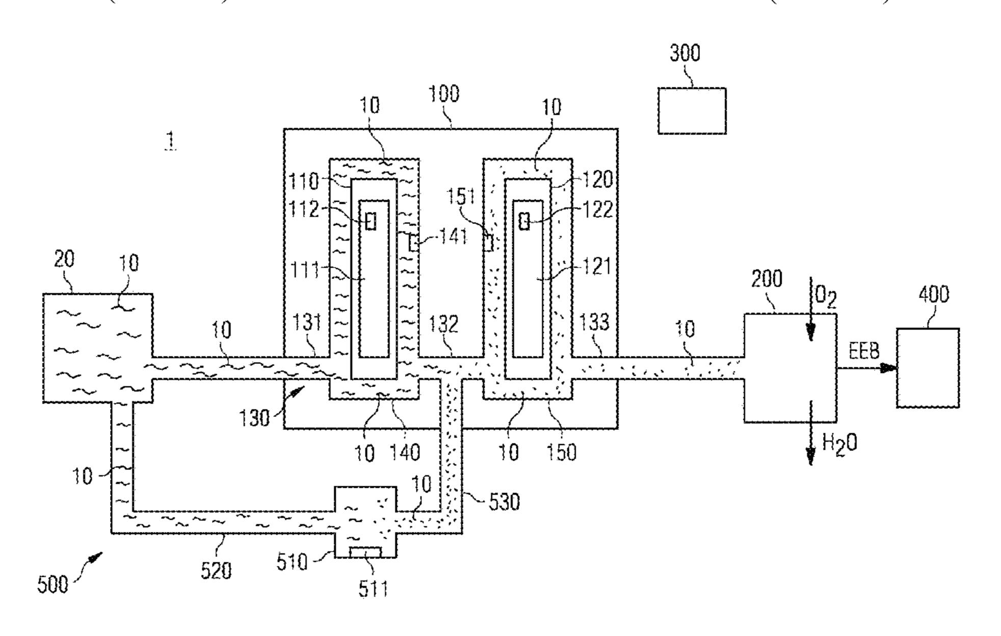
in gaseous form to a further component of the machine to cool the component, utilizing the heating enthalpy of the coolant. The now heated coolant is fed to the fuel cell, which uses the coolant supplied to the fuel cell as an operating medium and reacts it.
