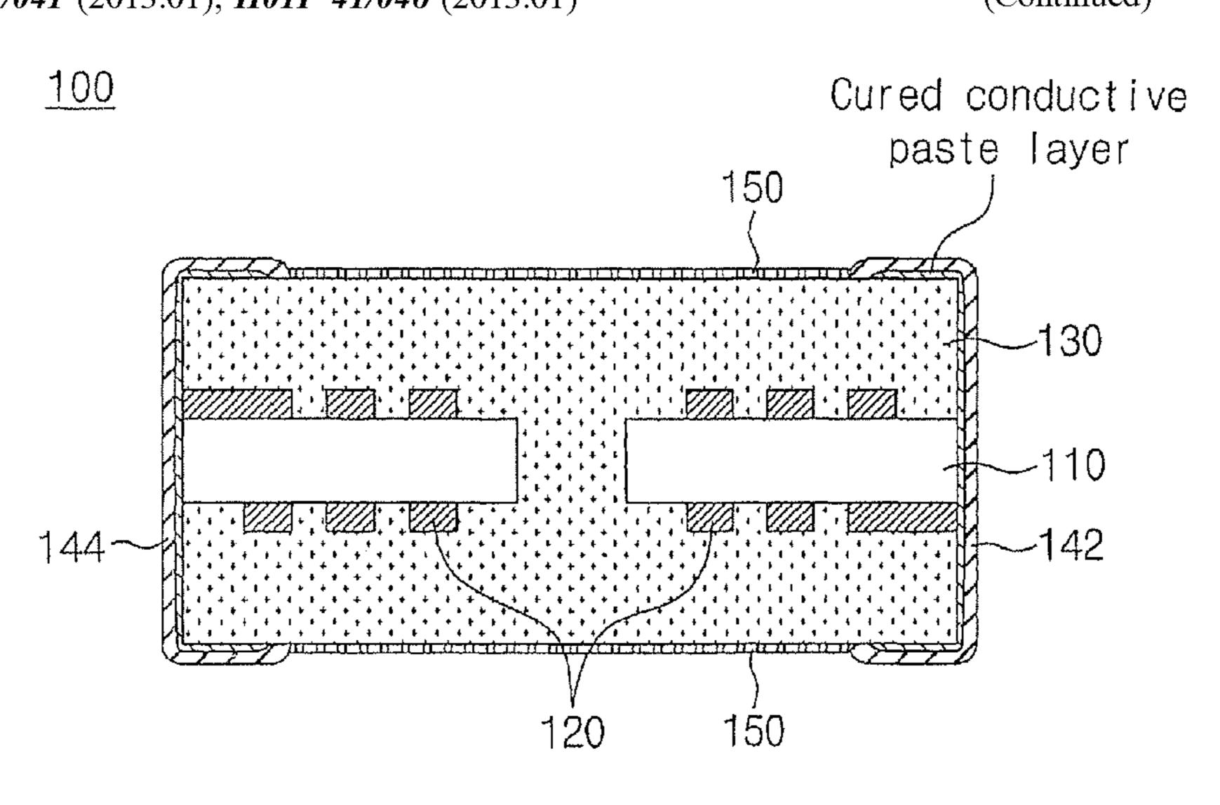
layer covering the magnetic body between the first external electrode and the second external electrode.
