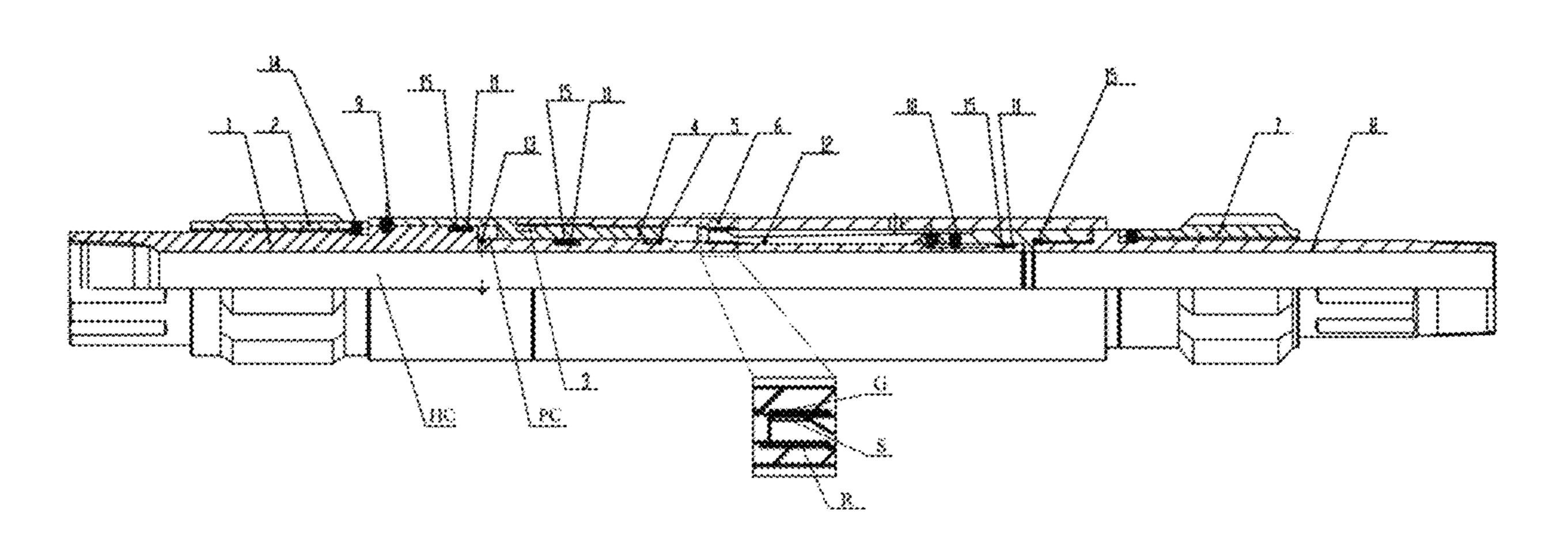
to limit the pawl. A releasing sleeve upper portion is arranged between the releasing sleeve and the upper joint, one end of the releasing sleeve upper portion is inserted into the releasing sleeve, and the other end is sleeved on an outer portion of the upper joint and connected to the upper joint via a start pin.
