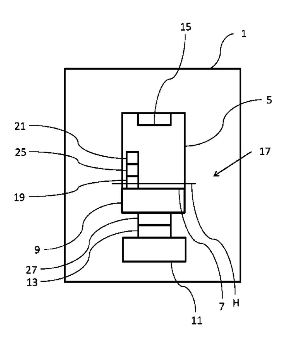
said build surface of said build plate, wherein said homing device is designed for moving said build surface to said home position until a measured force for displacing said homing member is within a pre-determined range. Method for producing an object by means of additive manufacturing.
