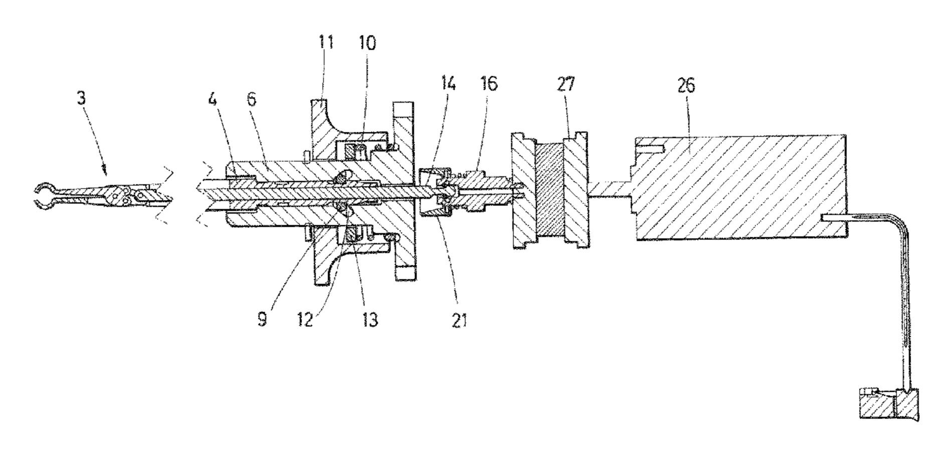
first tool part. The tool coupling further includes a first base part for detachably retaining the first tool part and a second base part movable in relation to the first base part for detachably retaining the second tool part. The first base part has a pusher movable in relation to the first base part for detaching the first tool part and the second base part has a cap movable in relation to the second base part for detaching the second tool part.
