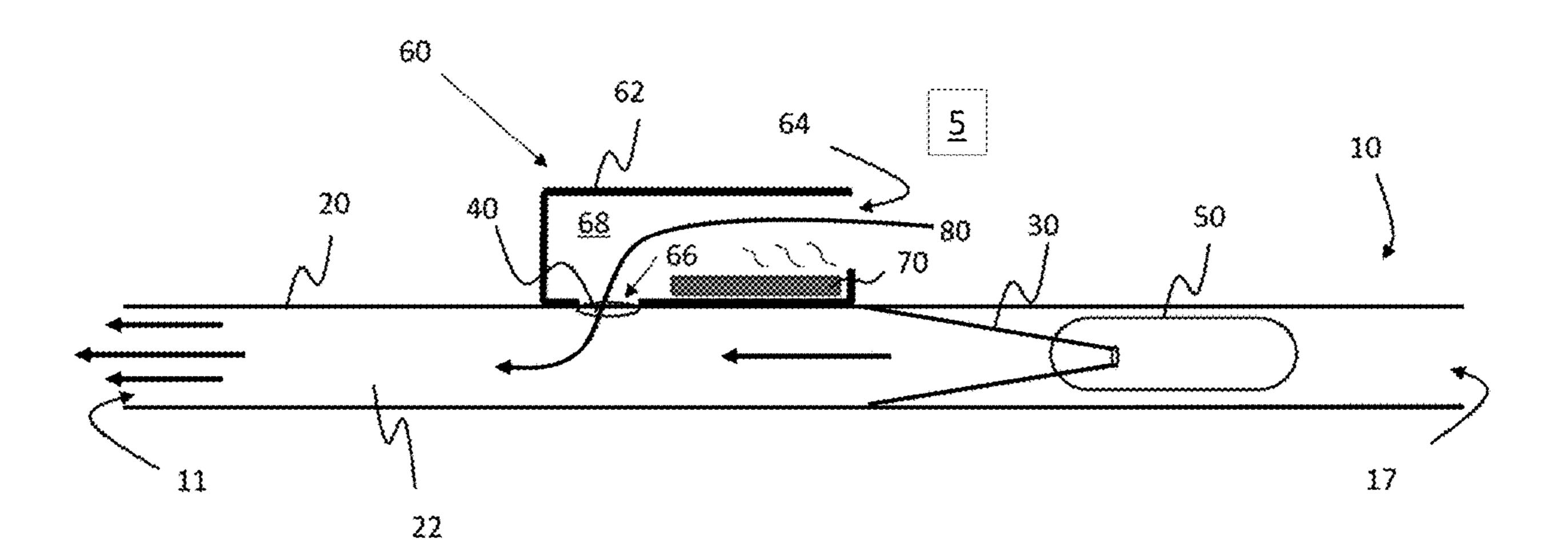
aligns with the at least one air inlet of the inhaler to form an airflow path through the device and into the inhaler.
