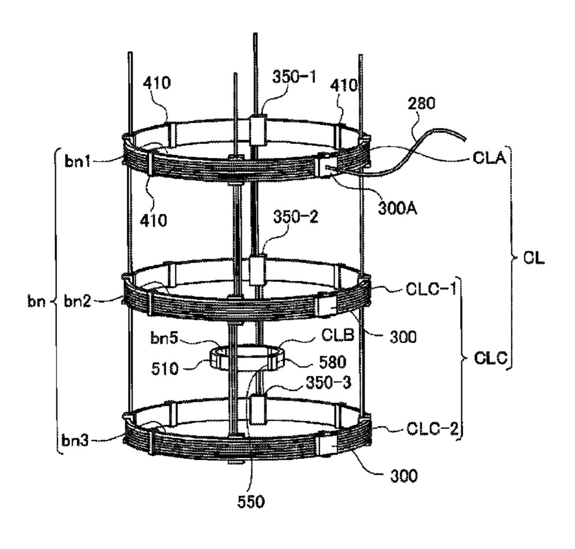
periphery along an inner periphery of the annular transmitting coil, and supporting the transmitting coil from the inner space, a power transmitting unit configured to supply A/C power to the power transmitting coil, and a capacitor connected to the transmitting coil, and forming a resonance circuit resonating together with the transmitting coil.
