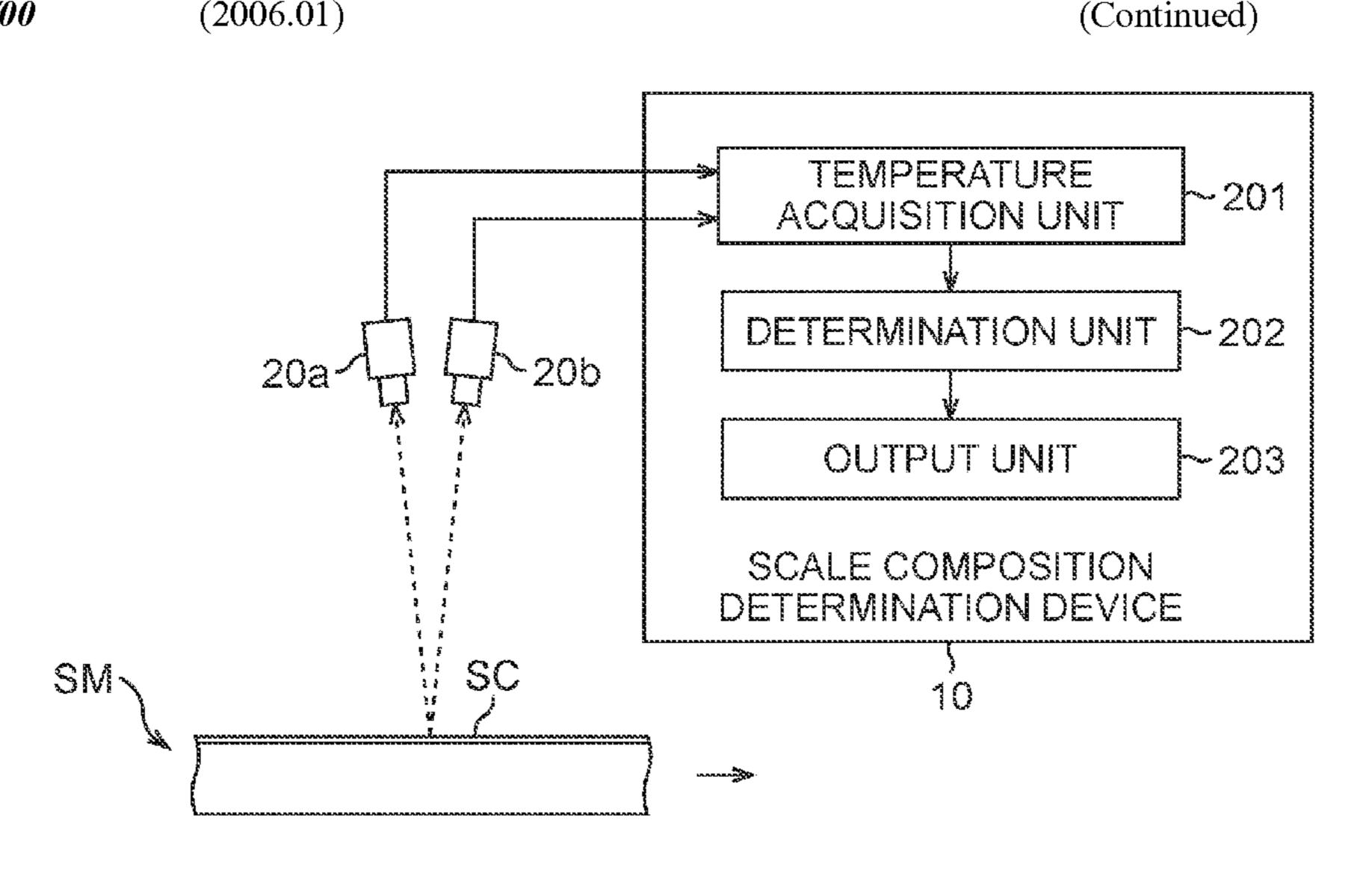
or more than a predetermined temperature, and determines that  $Fe_2O_3$  has not been generated in the outermost layer of the scale (SC) in the case where the absolute value of the difference between the temperatures of the steel material SM measured by the radiation thermometers (20a, 20b) is not equal to or more than the predetermined temperature.
