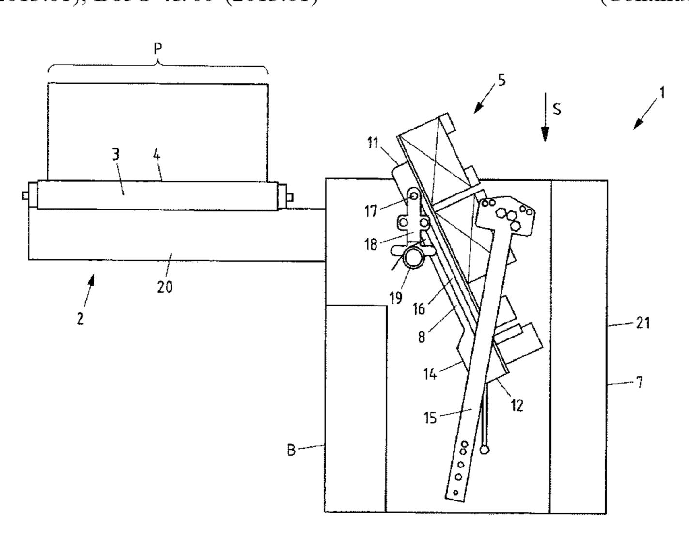
apparatus having such a conveying apparatus and having an applicator for applying a label to the respective product.
