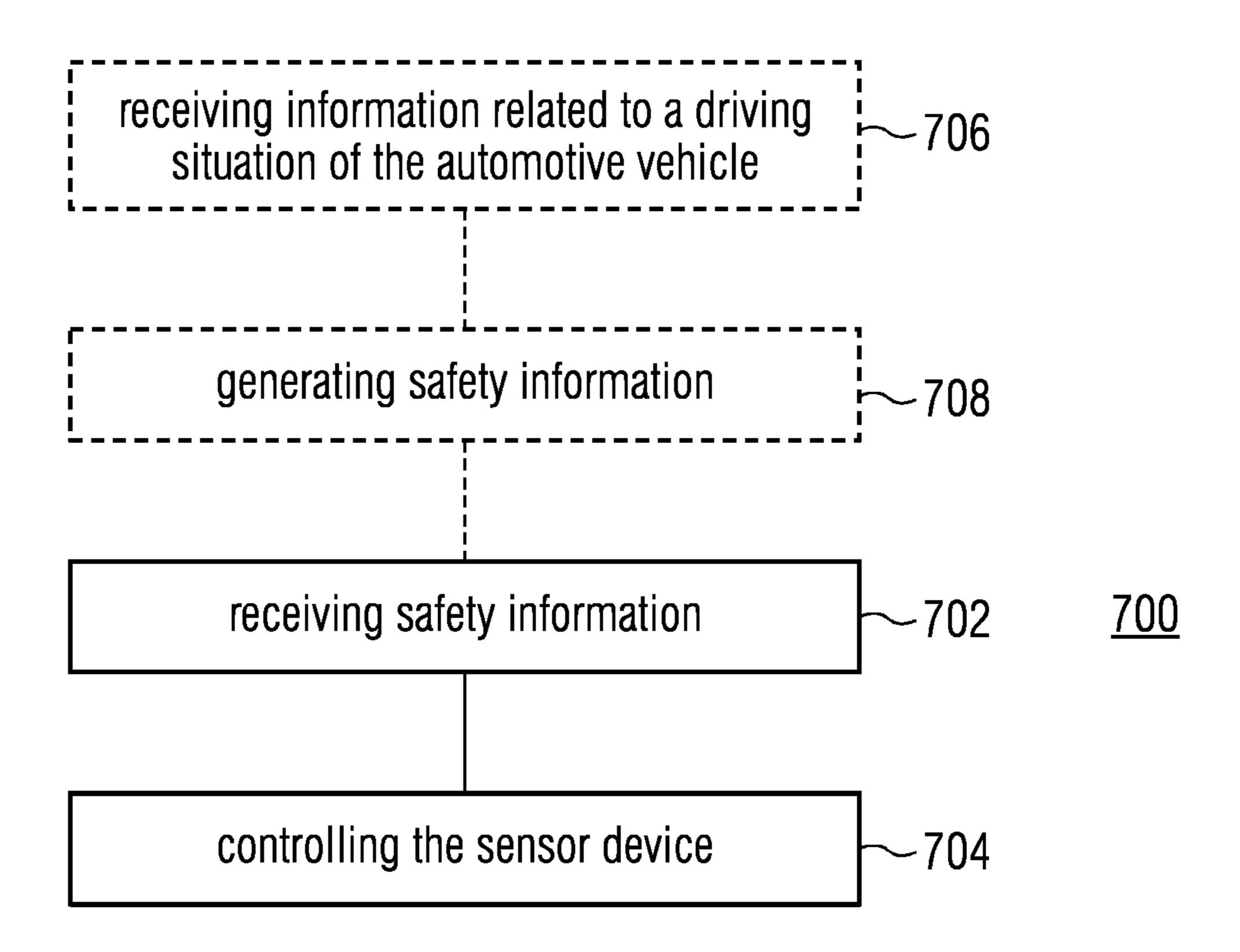
APPARATUS AND METHOD FOR CONTROLLING A SENSOR DEVICE OF AN OBJECT'S SAFETY SYSTEM, CONTROL SYSTEM FOR AN AUTOMOTIVE VEHICLE, AND SENSOR DEVICE FOR A SAFETY SYSTEM OF AN AUTOMOTIVE VEHICLE
