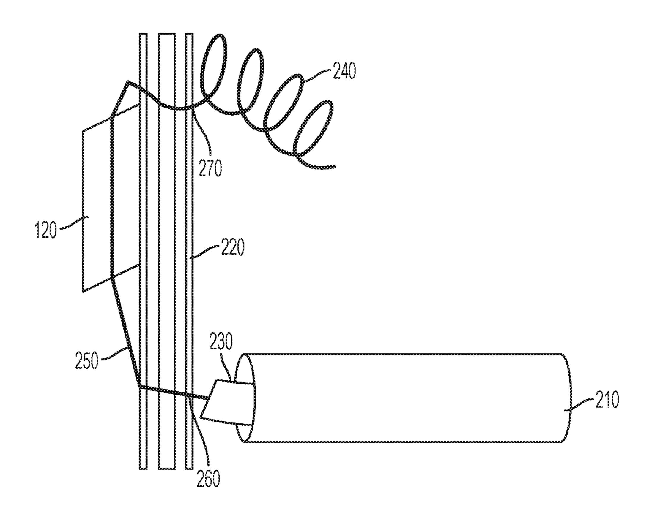
AN PERICARDIAL PAD IS DEPLOYED-ALSO PRE-LOADED ON PERINEEDLE-THIS KEEPS THE TENSION ON THE WIRE AND KEEPS THE COIL IN CLOSE CONTACT WITH THE INSIDE OF THE PERICARDIUM
