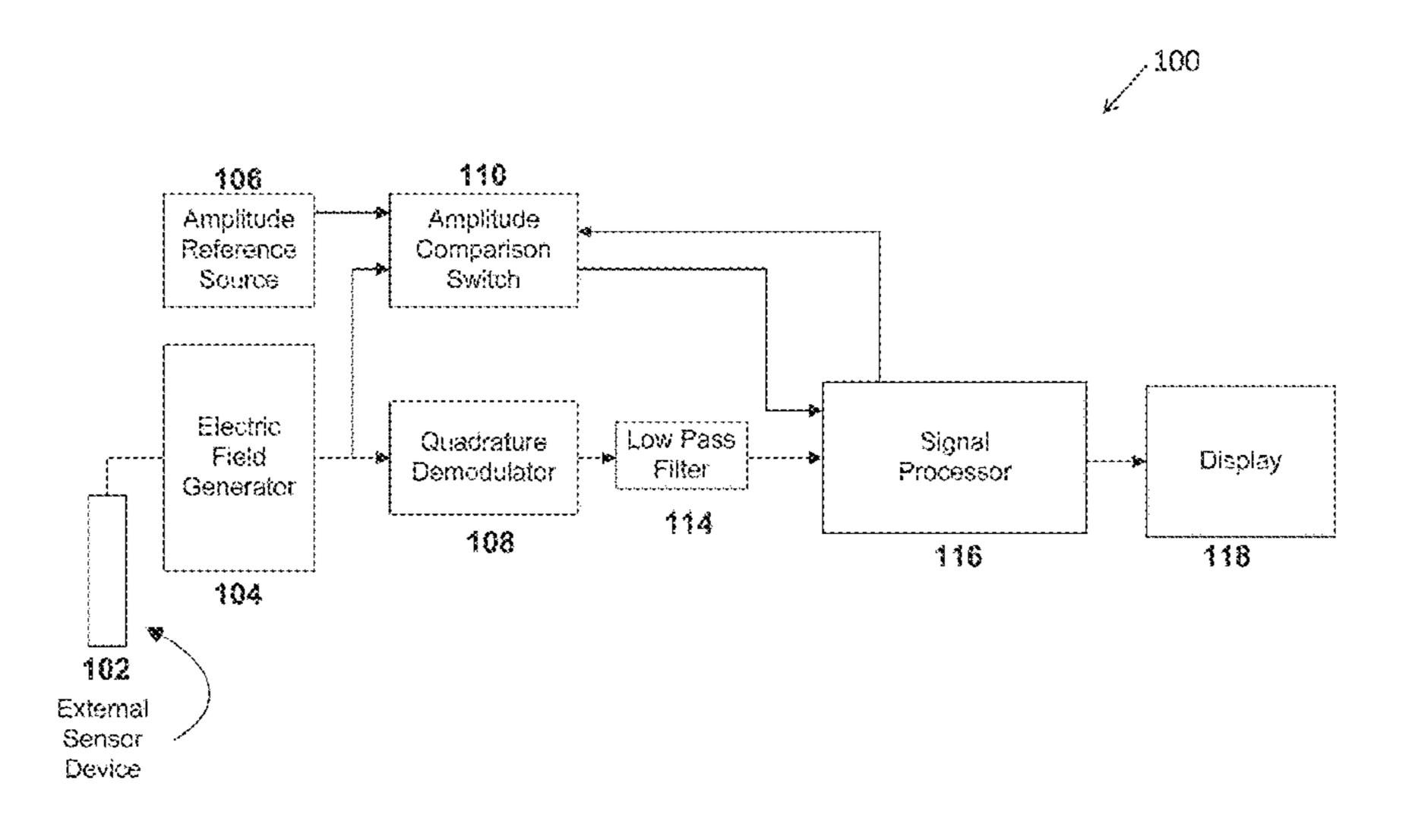
output of the electric field generator. The system includes a signal processor configured to analyze the changes of the amplitude and frequency of the output of the electric field generator.
