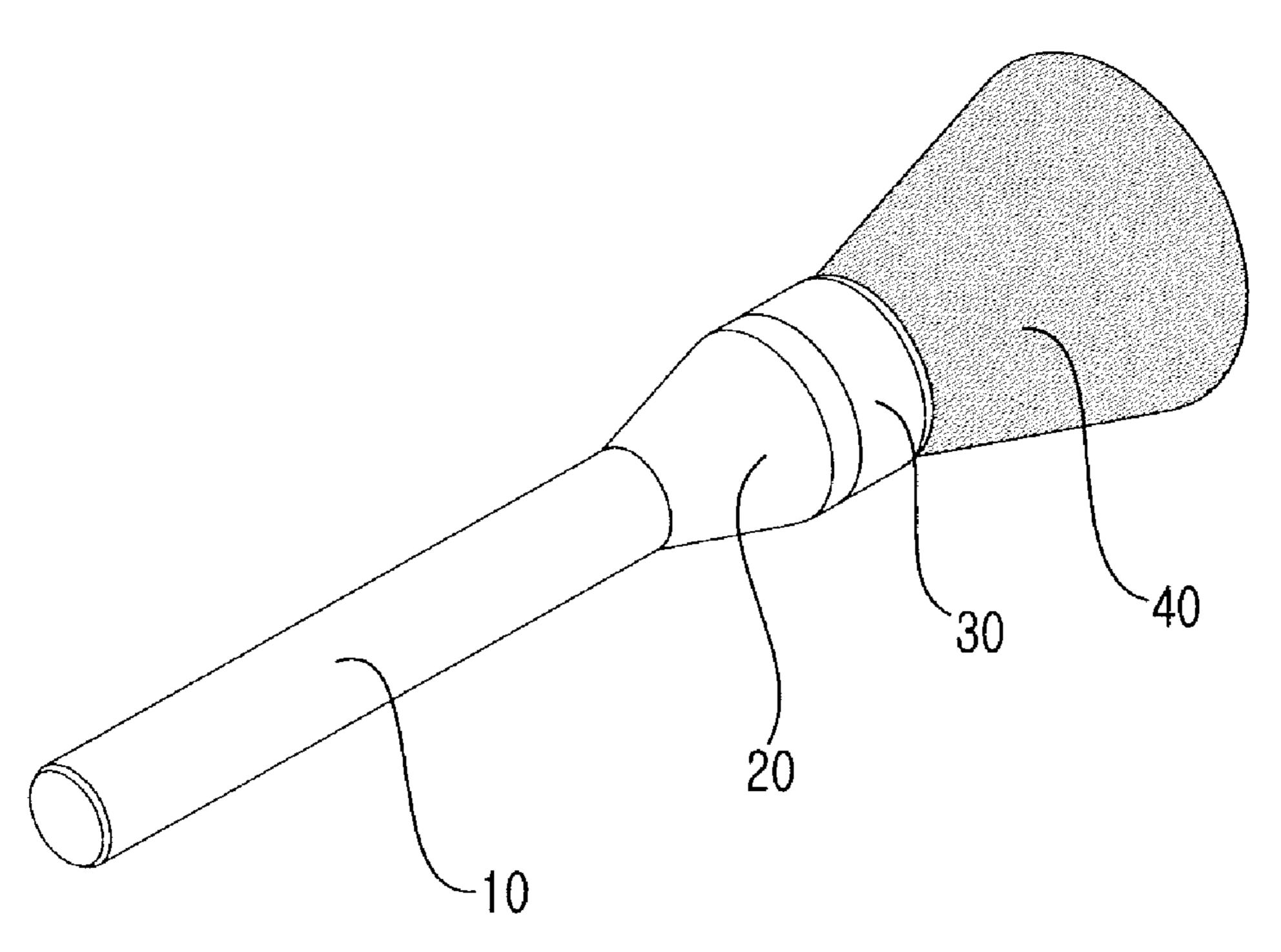
end part of the handle is detachably coupled; a brush fixing ring made of the biodegradable resin, and having the rear end thereof to which the front end part of the neck part is detachably coupled; and a head part inserted into a rear end part of the brush fixing ring and fixed therein, and having a bristle bundle integrally implanted on the front surface thereof.
