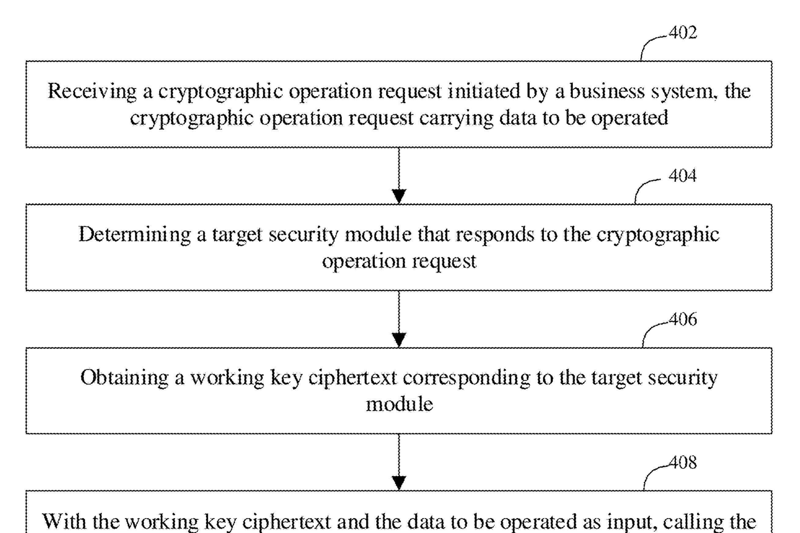
target security module to obtain an operation result returned by the target security module and send the operation result to the business system
