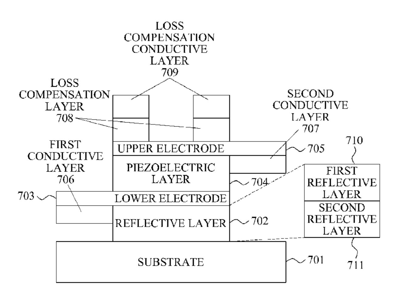
includes an upper electrode formed on the piezoelectric layer, and a conductive layer formed on the upper electrode or the lower electrode.
