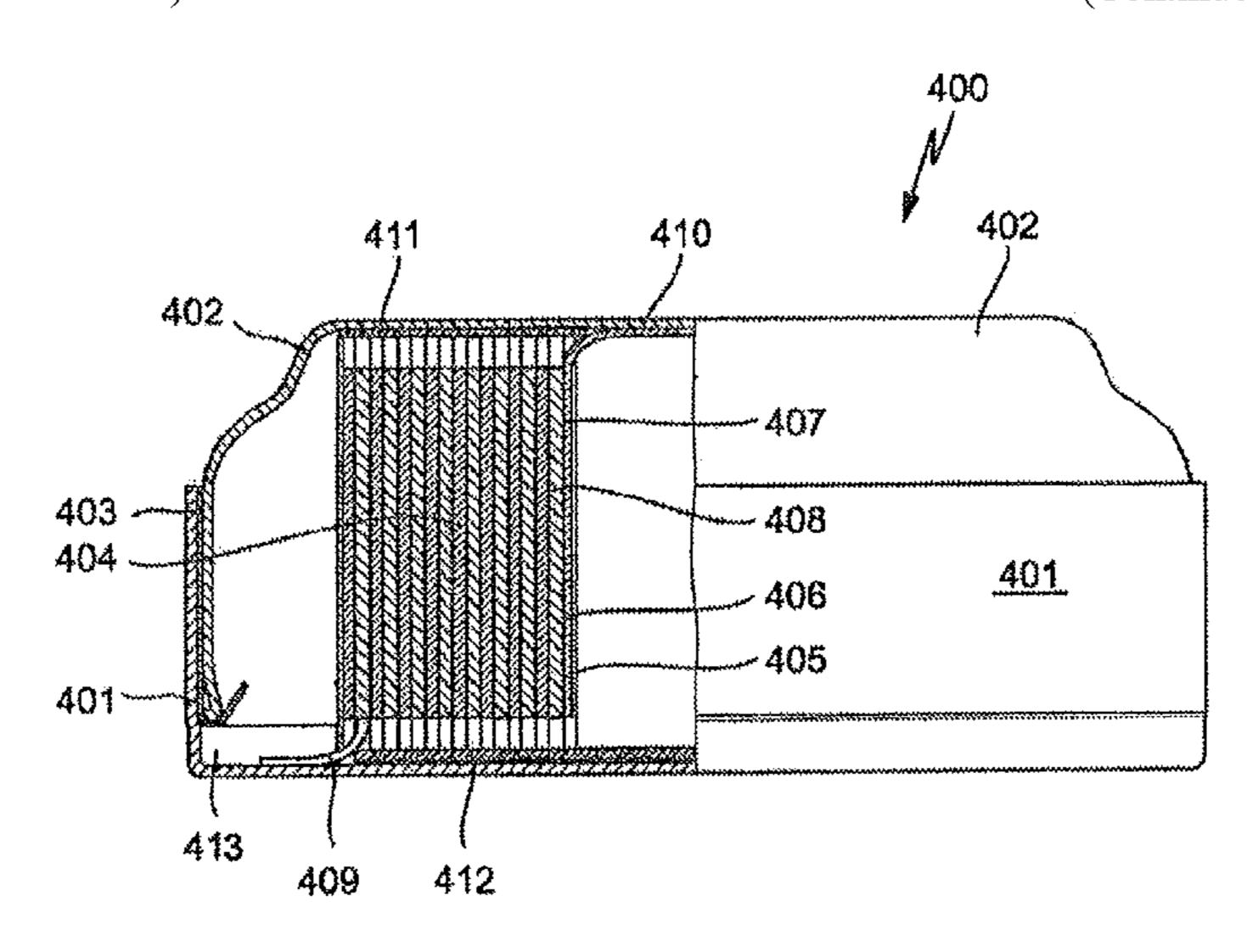
electrode formed from a second metallic film or mesh coated with a second electrode material, and a separator disposed between the positive electrode and the negative electrode. The first metallic film or mesh is bent such that at least a portion extends out of the electrode-separator assembly winding and wherein at least a first part of the portion is not covered with the first electrode material.
