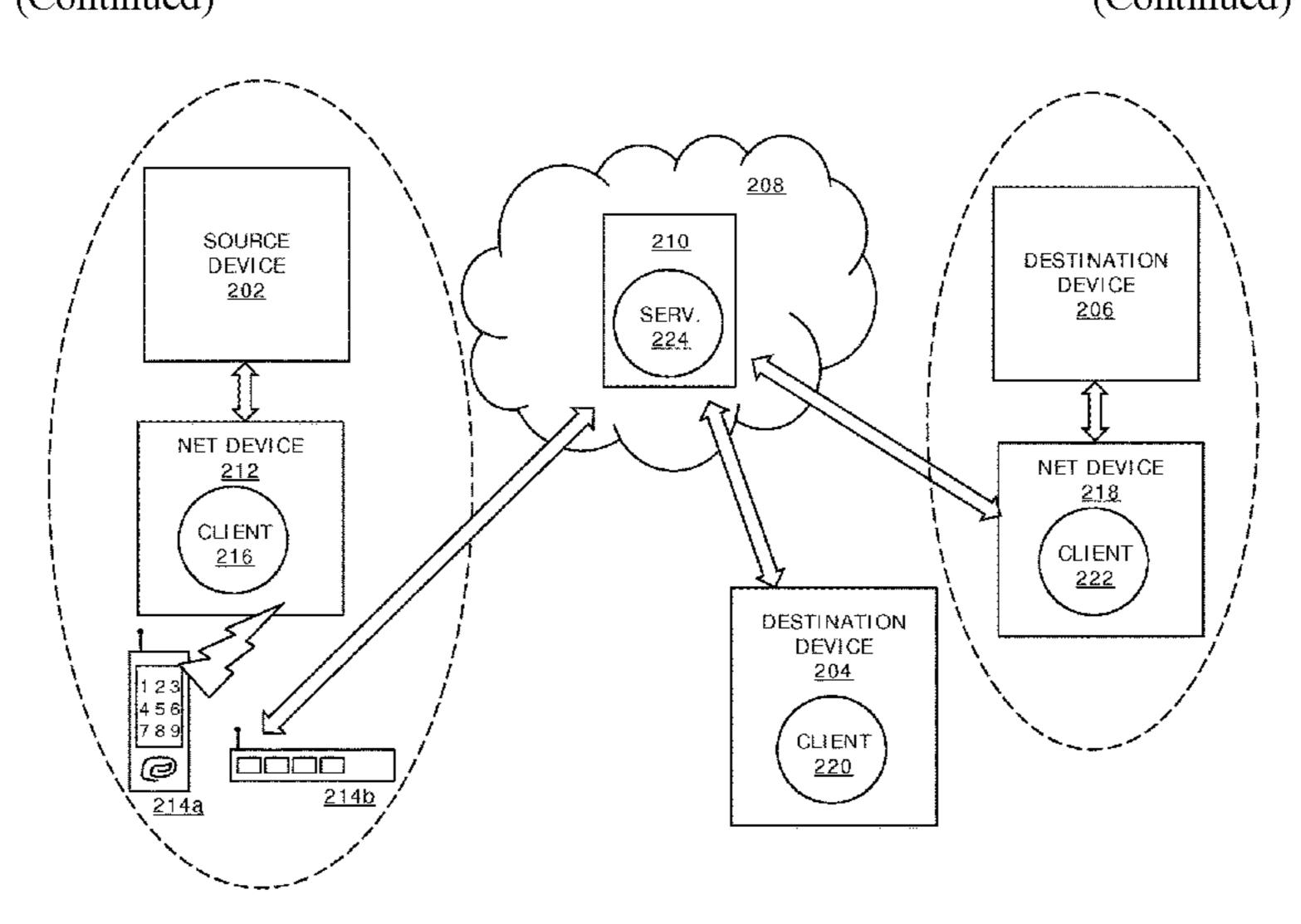
nication network. The source client is configured to communicate the data to the destination device, by relaying the data through the network node service, when the destination client is connected to the network node service.
