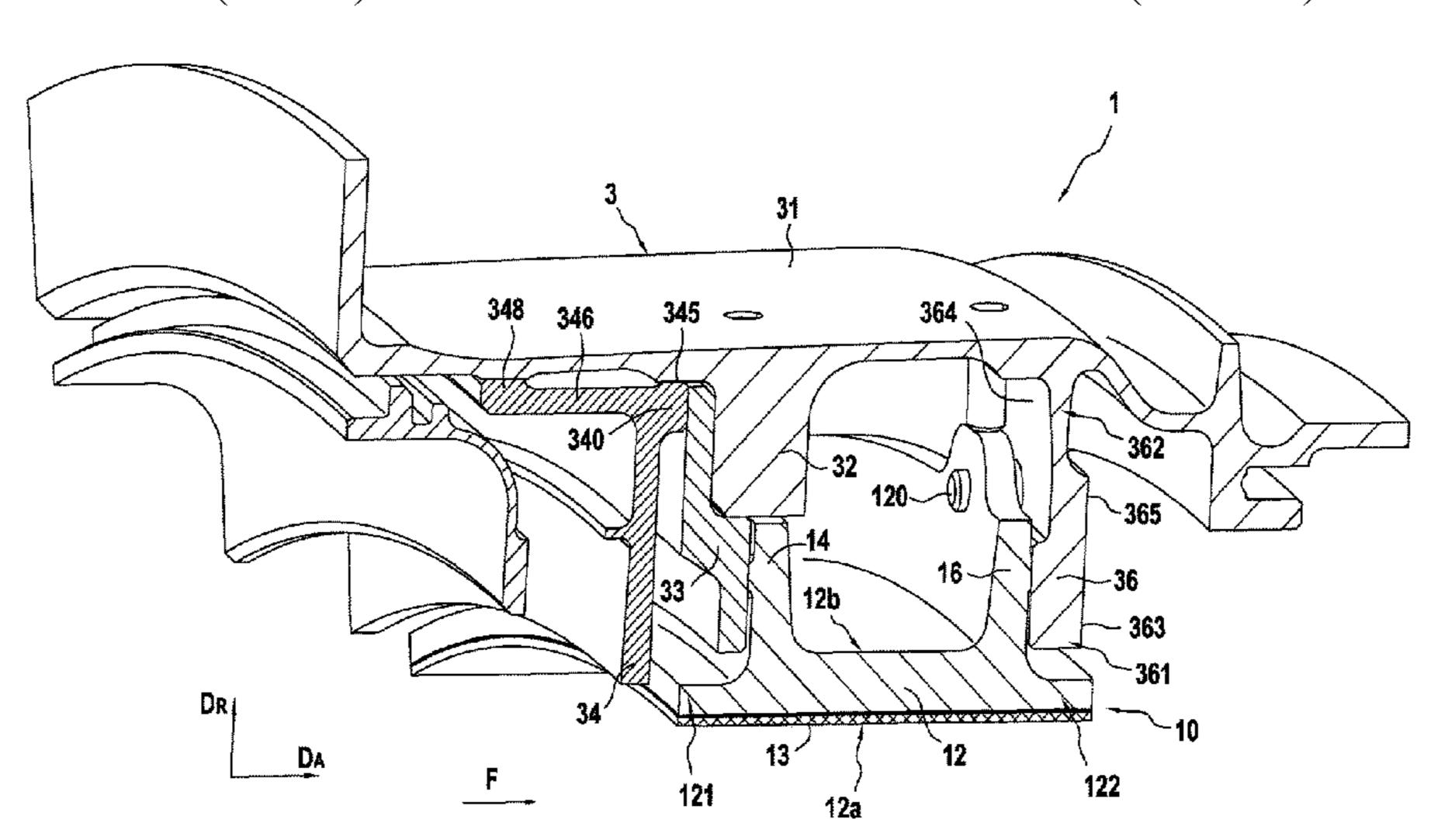
to the first radial clamp, the second annular flange including a support shroud projecting upstream in the axial direction and having a radial support in contact with the central shroud.
